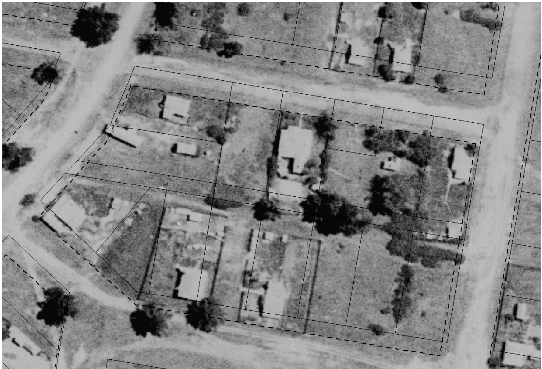
Figure 6.1 Comparison of Current DCDB to Adjusted DCDB (Reproduced with permission from Armidale Dumaresq Council)
