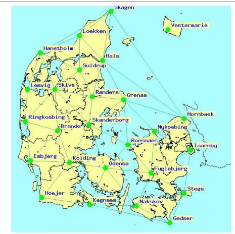
Figure 2.2: GPSnet.dk Coverage Area in Denmark (*GPSnet.dk Coverage Map Denmark* 2005)
