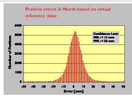
Figure 2.3: The expected Horizontal accuracies of GPSnet.dk (*The idea behind GPSnet.dk* is simple - VRS is ingenious 2005)
