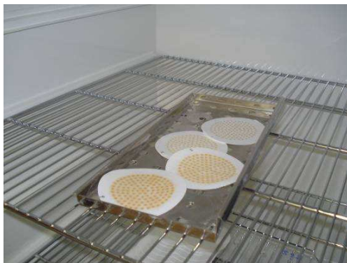
Figure 3.4 TSS test procedure showing (a) TSS filter apparatus and samples, (b) Drying oven, (c) Desiccator and samples, (d) Analytical balance
