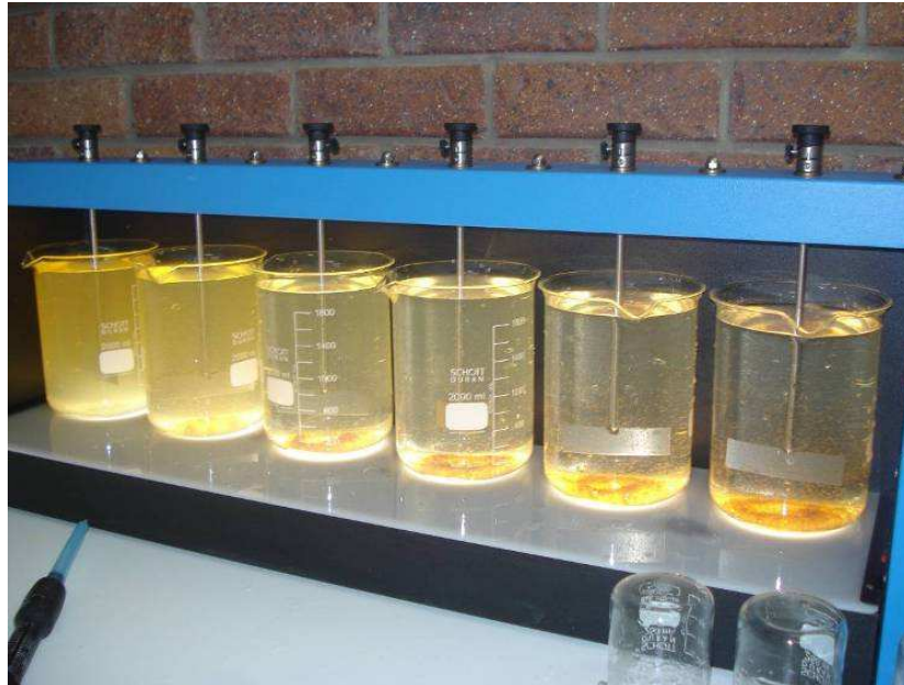
Figure 4.5 Jar testing of East Creek stormwater. Dosages range from 6.0mg/L (far left jar) to 11.0mg/l (far right jar)
