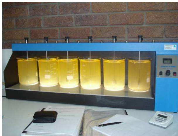
Figure 3.5 A Phipps & Bird Model PB – 700 Jar Tester with six 2000mL samples.
