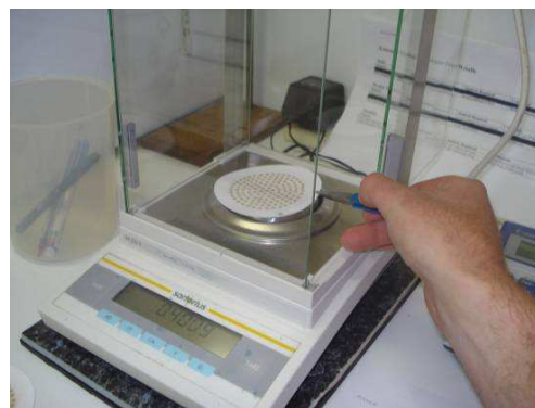
Figure 3.4 TSS test procedure showing (a) TSS filter apparatus and samples, (b) Drying oven, (c) Desiccator and samples, (d) Analytical balance
