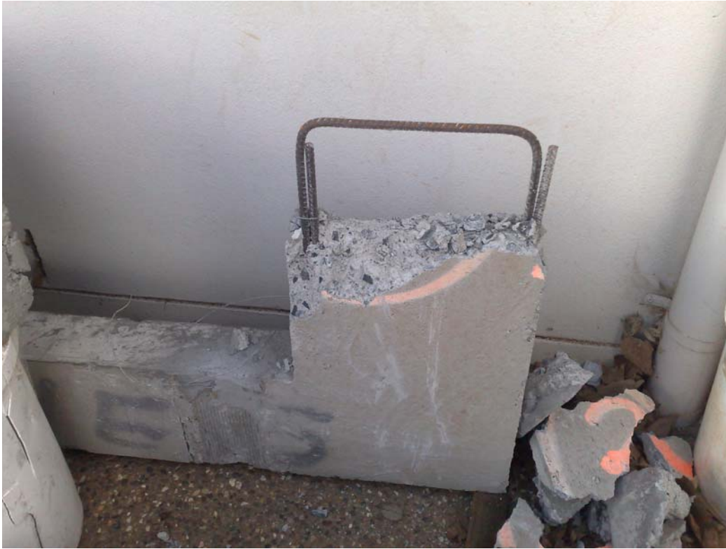
Figure 5.2 Destruction loading results to Beam 2.
