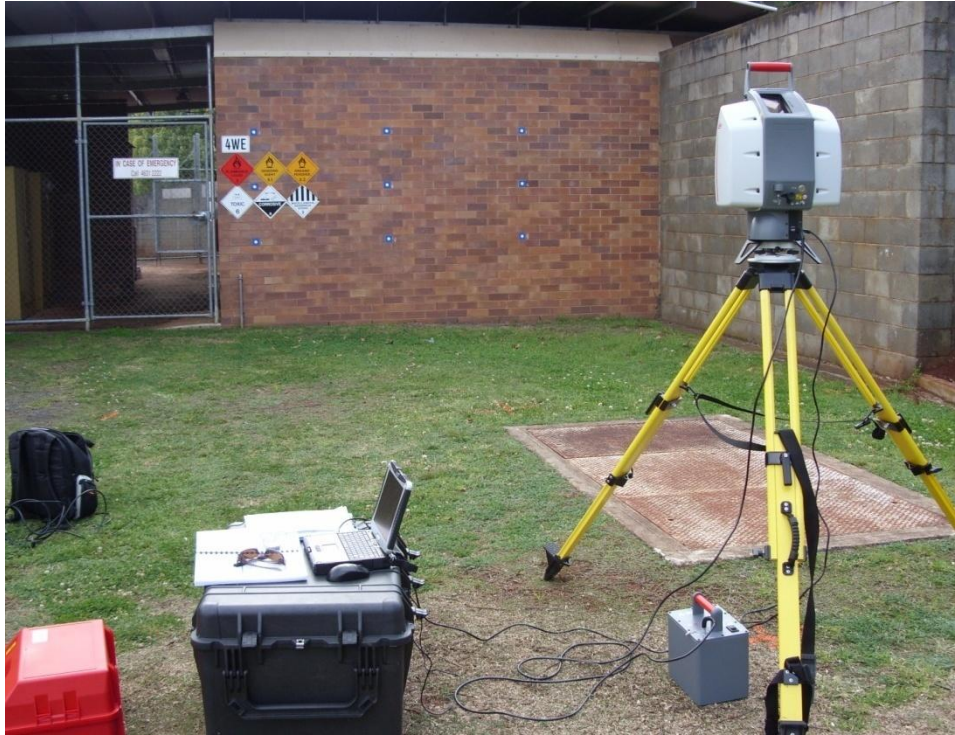
Figure 3.6-2: Testing procedure set-up for the laser scanner
