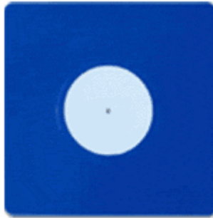
Figure 2.2-6: The HDS targets used as control points.
