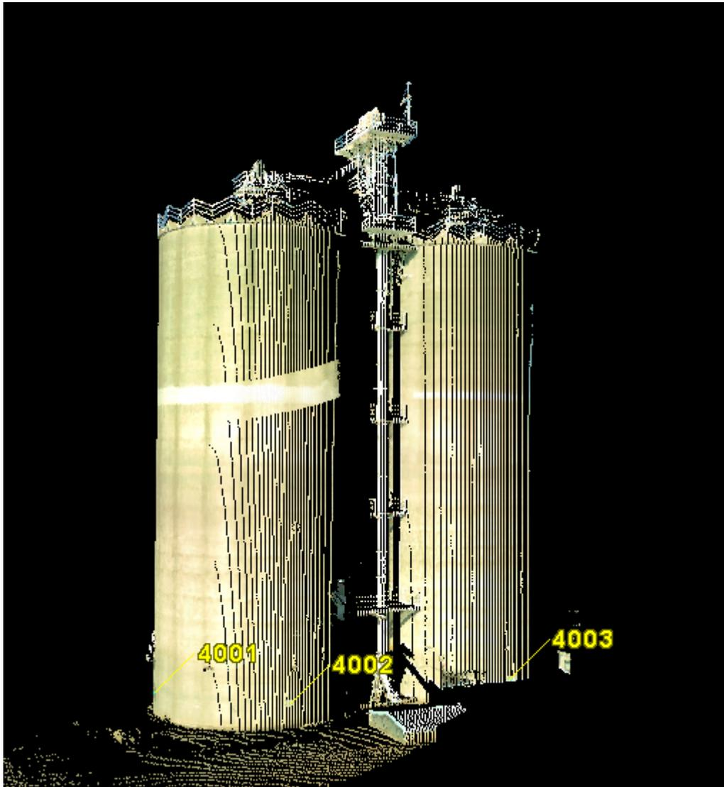
**Figure 4.3: Scan from survey control station 1002**
