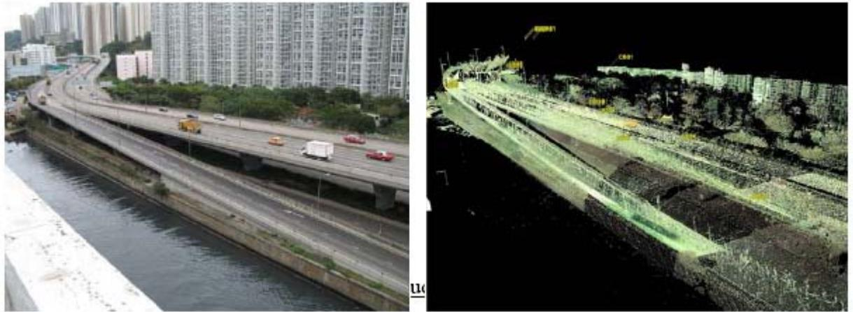
**Figure 2.3: Picture of area to be laser scanned and the point cloud**
