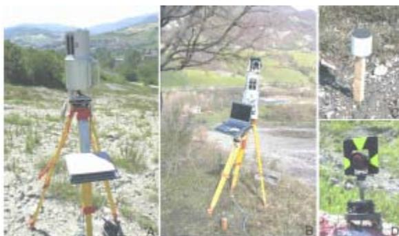
**Figure 2.2: Using laser scanning to monitor land slides.**
