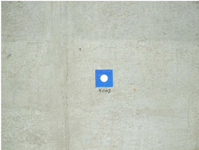
**Figure 3.3: Leica HDS target**
