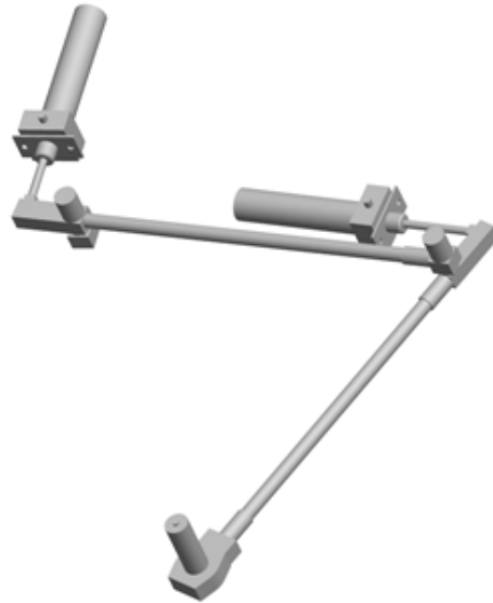
Figure 3.12: Linear Pneumatic Implementation
