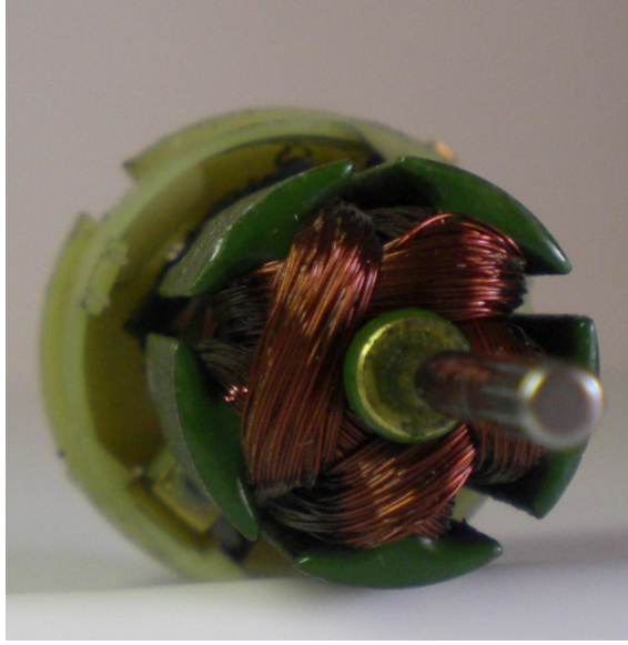
Fig. 2.2: A permanent magnet DC motor winding with a coil pitch of 2 slots.
