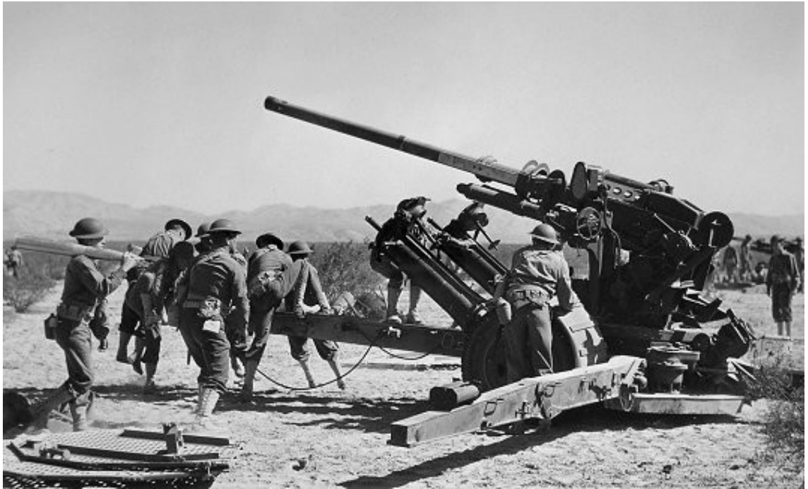
Fig. 1.4: 90mm anti-aircraft gun M1 on mount M1 (Brooks 2008)
