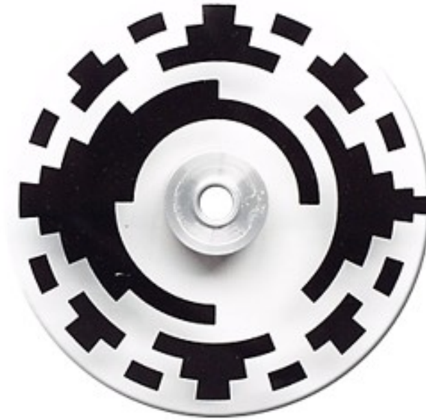
Fig. 2.14: Gray code pattern of dark tracks on the disc. (Feedback Instruments Limited 1999)
