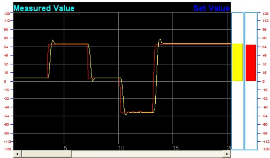
Fig. 3.13: Feedback Instruments tutorial software display showing the response of the servo to various steps in input.
