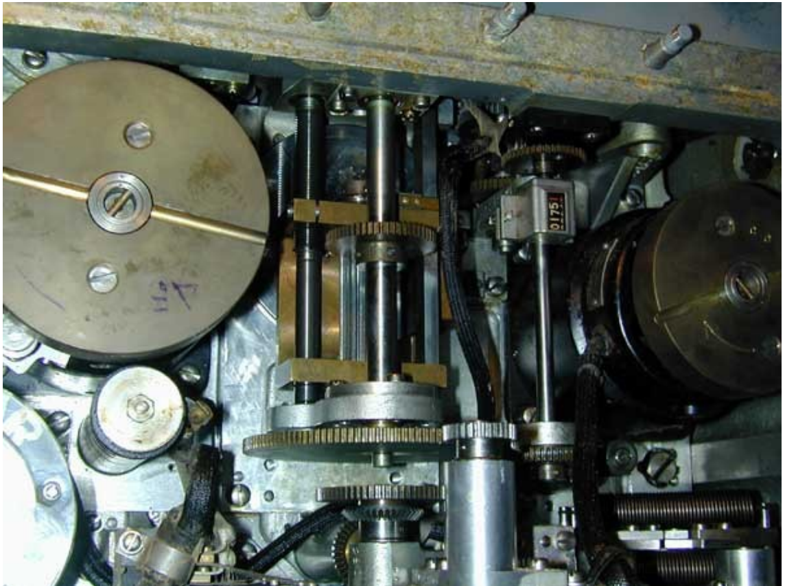
Fig. 1.5: Mechanical integrator inside the torpedo data computer of the USS Cod submarine (USS COD Home Port 2007)
