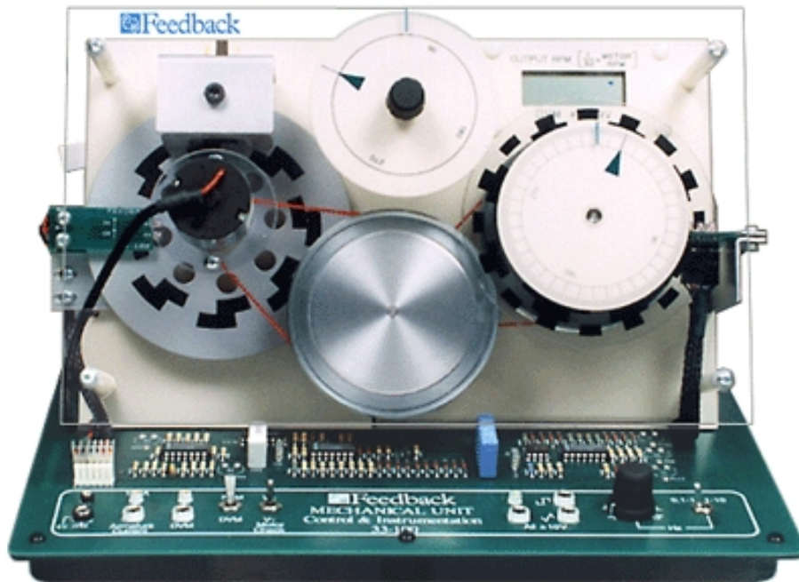
Fig. 1.2: Feedback Instruments Servo Fundamentals Trainer mechanical unit (Feedback Instruments Limited 1999)
