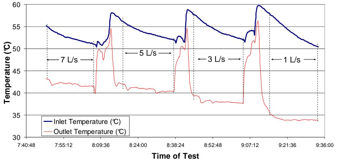
**Figure 6.5** Pipe in-water test results indicating inlet and outlet temperatures as well as the 20 minute regions of varied flowrates for the COPPER pipe material.
