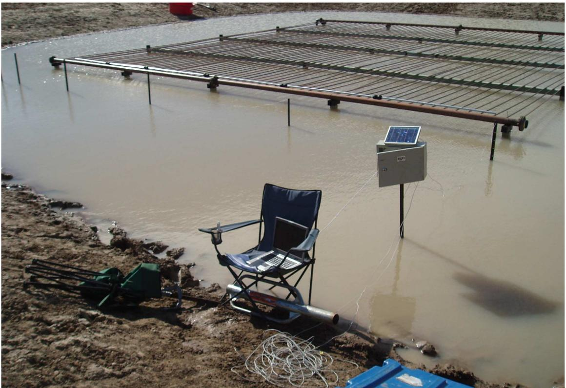
**Figure 5.3** Water test apparatus with submerged test material fixed to steel posts
