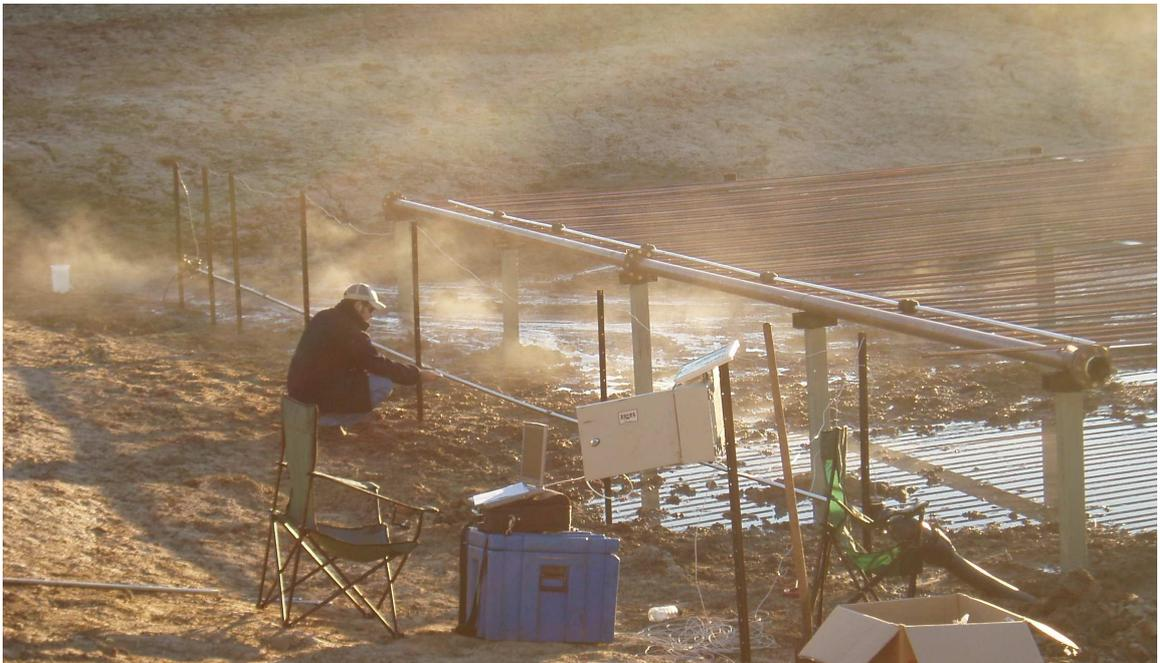
**Figure 5.2** Data logger and manual readings during pipe in air test
