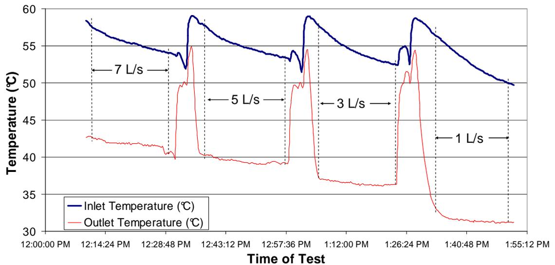
**Figure 6.4** Pipe in-water test results indicating inlet and outlet temperatures as well as the 20 minute regions of varied flowrates for the ALUMINIUM pipe material.
