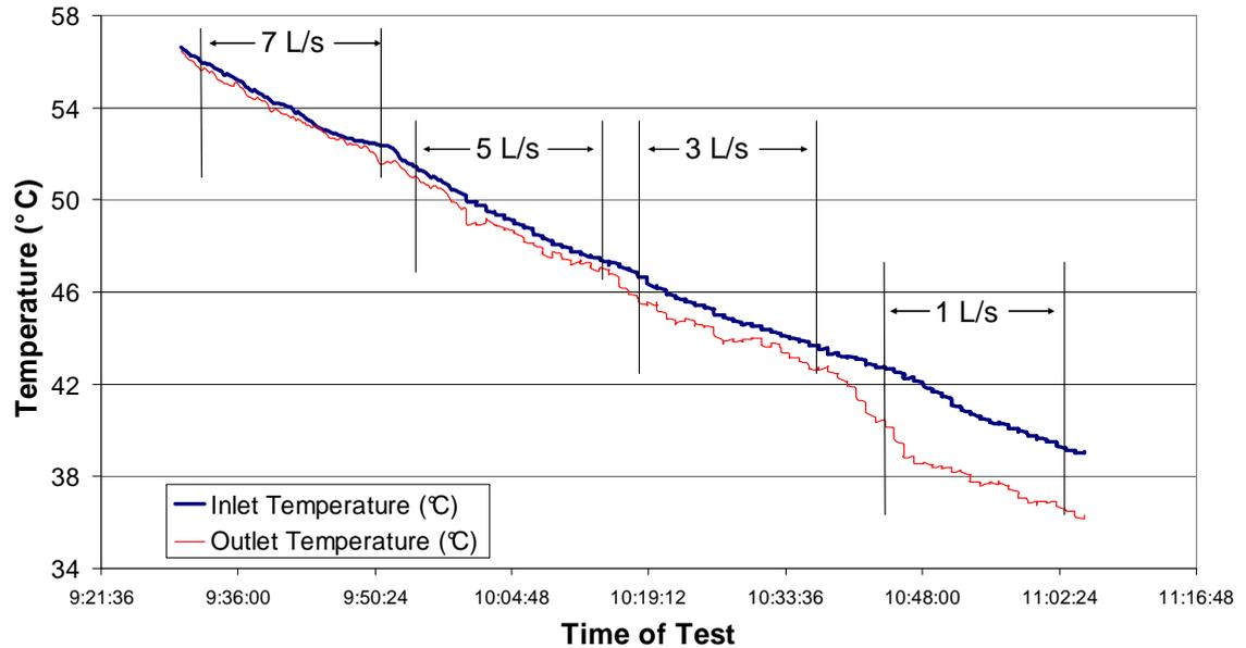
**Figure 6.2** Pipe in-air test results indicating inlet and outlet temperatures as well as the 20 minute regions of varied flowrates for the COPPER pipe material.
