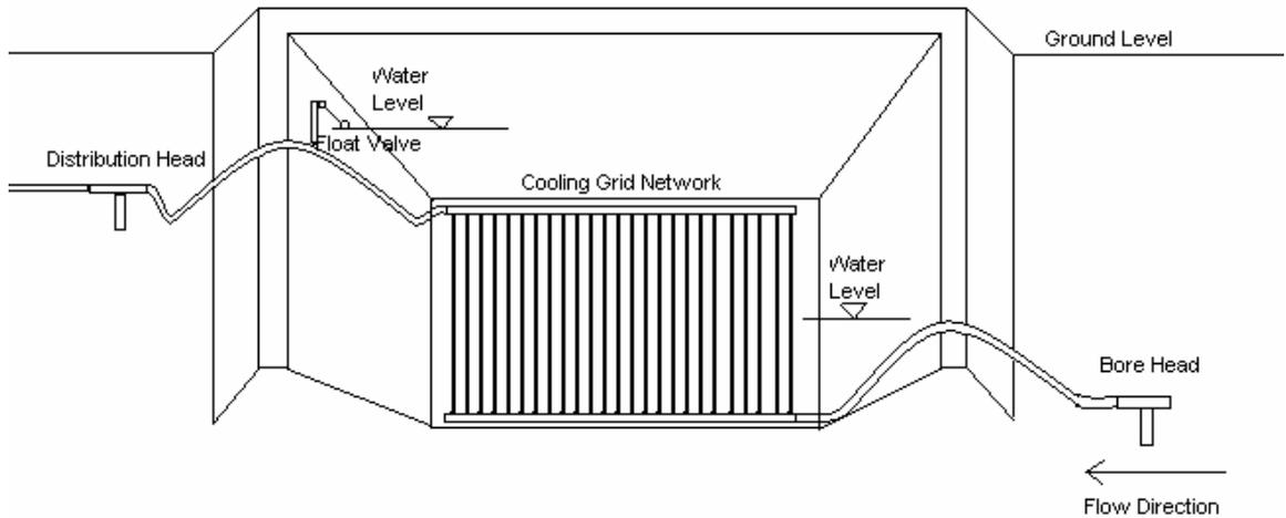
**Figure 1.1** Schematic of Typical Cooling Grid
