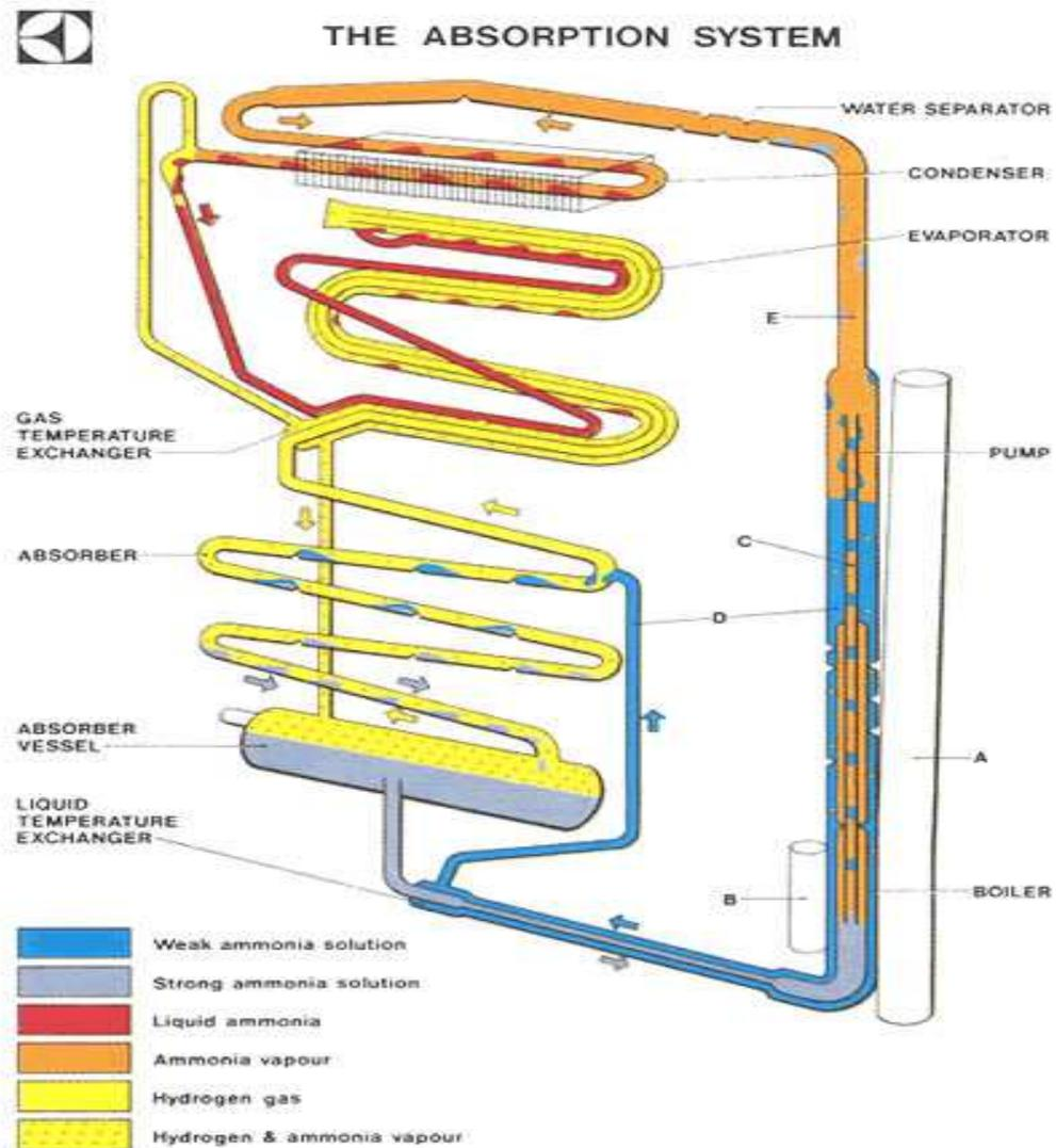
**Figure 3.1** Gas Absorption System. *Source: Lehman's Gas Refrigerators, 2007*
