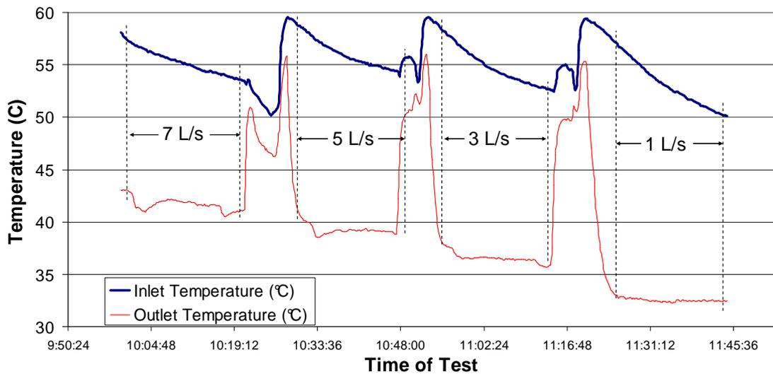
**Figure 6.6** Pipe in-water test results indicating inlet and outlet temperatures as well as the 20 minute regions of varied flowrates for the STAINLESS STEEL pipe material.
