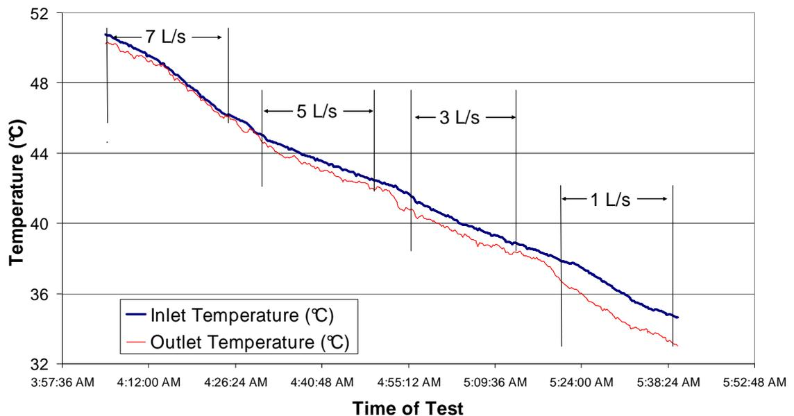
**Figure 6.1** Pipe in-air test results indicating inlet and outlet temperatures as well as the 20 minute regions of varied flowrates for the ALUMINIUM pipe material.
