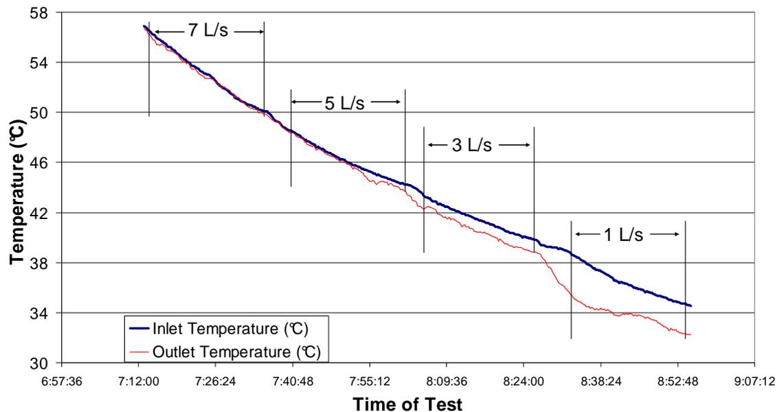
**Figure 6.3** Pipe in-air test results indicating inlet and outlet temperatures as well as the 20 minute regions of varied flowrates for the STAINLESS STEEL pipe material.
