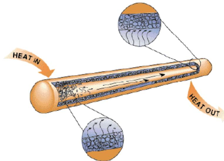
**Figure 3.2** Heat Pipe *Source: CheResources, 2008*
