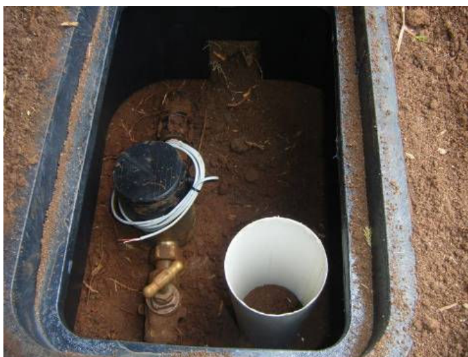
Figure 3-3 CT5-S meter(left) and installed(right)
