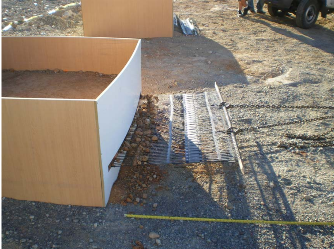
Figure 16 Pullout Load applied to Tensar Geogrid
