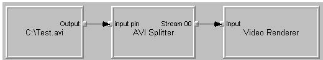
Figure 5.2: A Series of filters chained together with GraphEdit to decode and render a video file
