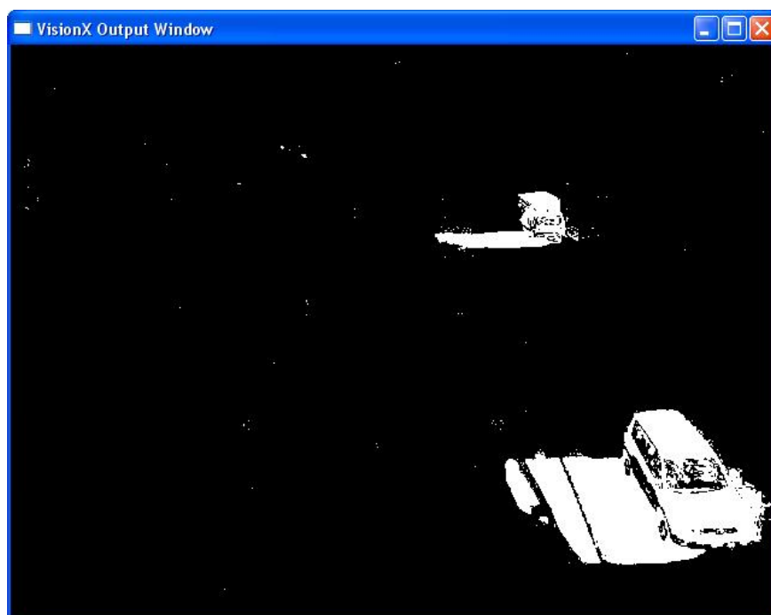
Figure 6.2: Result of Background Subtraction on a typical frame from traffic footage. The moving vehicles are clearly highlighted which generally makes it easier to implement object segmentation and identification.
