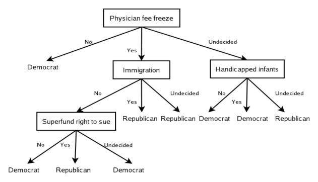
Figure 4.3: Decision tree for a subset of the voting data created using C4.5
