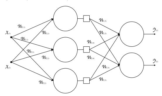
Figure 2.5: Example of a back propagation neural network
