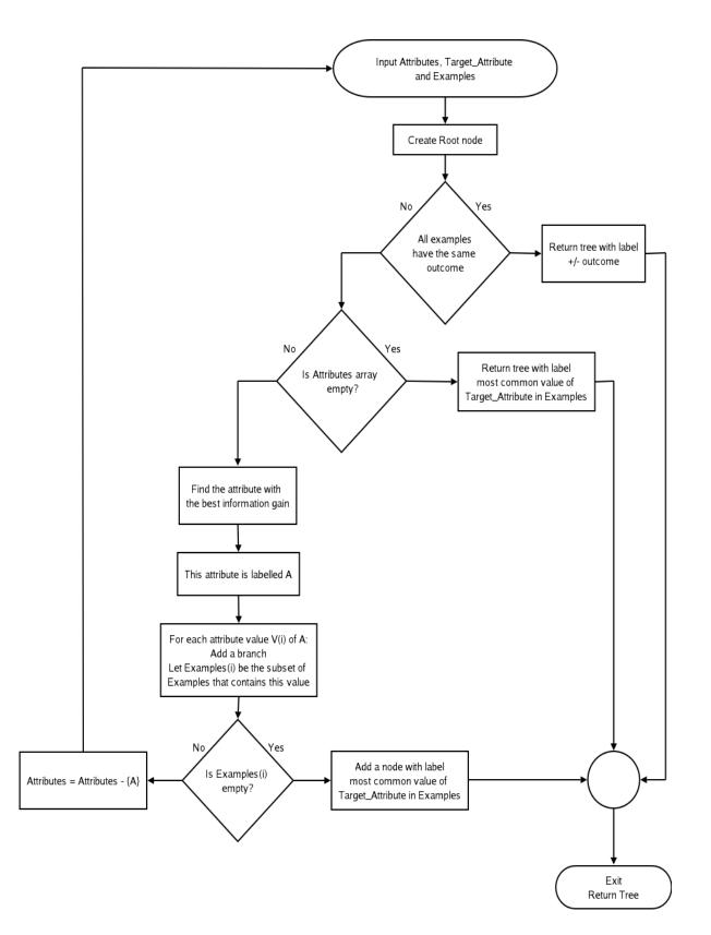
Figure 3.1: Flow chart representing the ID3 algorithm
