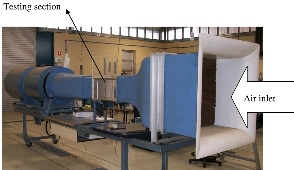
Figure 3.3a open circuit subsonic wind tunnel
