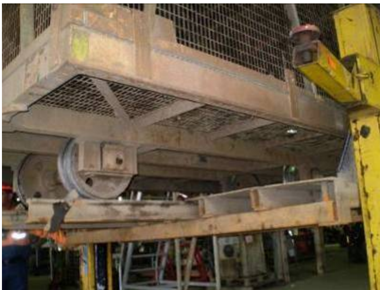
Figure 3.2 Underside of six tonne cane bin. (CSR Sugar)
