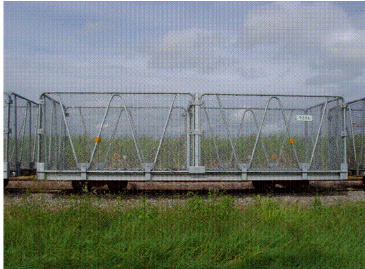
Figure 2.4 Eleven tonne cane bin. (CSR Sugar)
