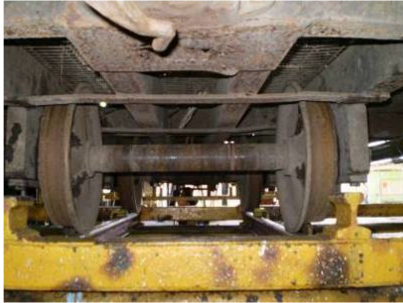
Figure 3.3 Four tonne cane bin wheel set. (CSR Sugar)
