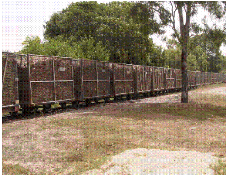
Figure 2.2 Four tonne cane bin. (CSR Sugar)
