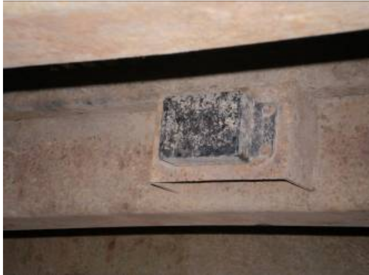
Figure 3.4 RFID tag mounted on the cane bin.
