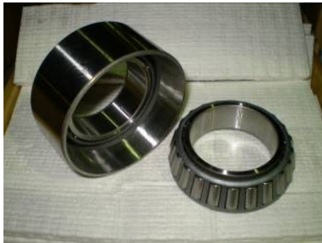
Figure 2.10 Currently utilised bearing.
