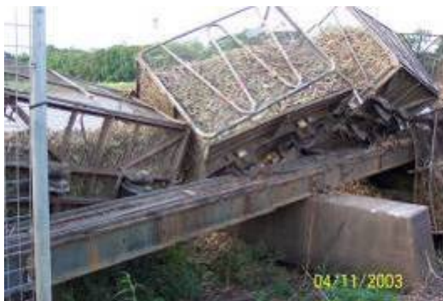
Figure 5.3 Example of a cane bin derailment. (CSR Sugar)
