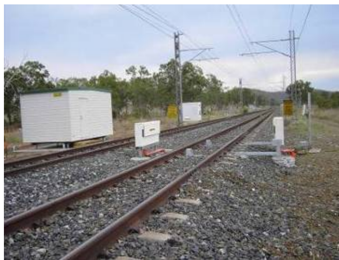
Figure 4.6 An operational RailBAM© system. (Vipac Engineers)
