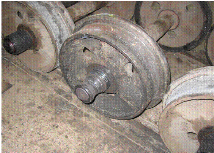
Figure 2.14 Failed bearing. (CSR Sugar)
