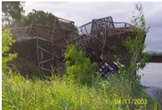
Figure 5.2 Example of a cane bin derailment. (CSR Sugar)
