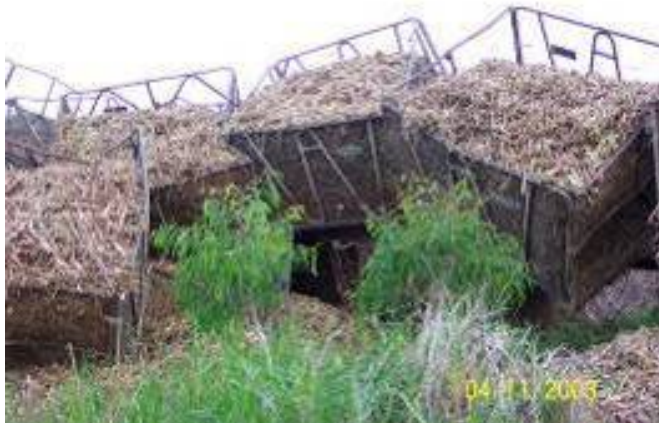
Figure 5.1 Example of a cane bin derailment. (CSR Sugar)
