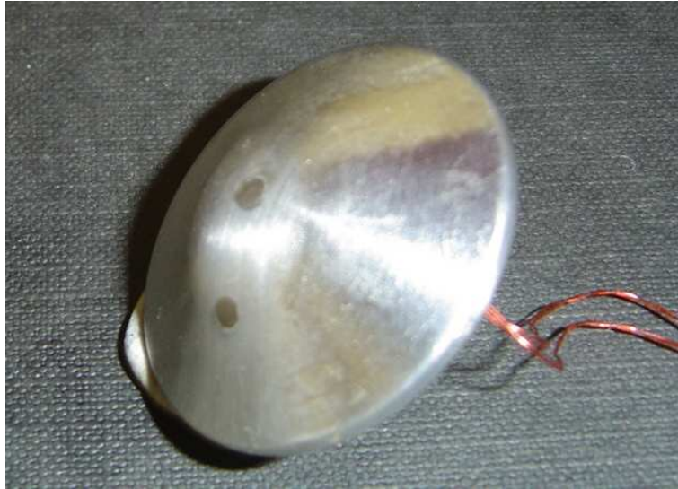
Figure 5.1: Photograph of the Model. Thermocouples are seen sitting flush with the model surface.
