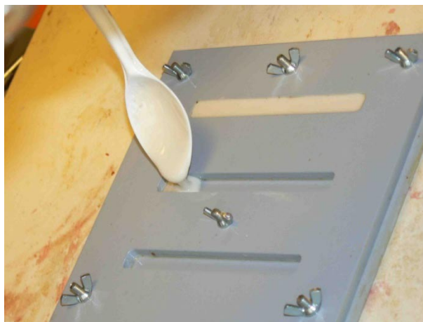
Figure 3.8: Pouring Composite Mixture into Moulds
