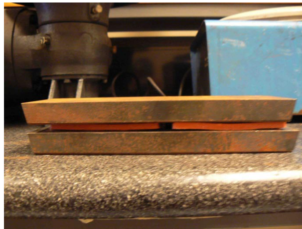
Figure 3.11: Specimen Support for Post Curing (Side View)
