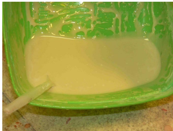
Figure 3.7: Mixed Phenolic Composite ready for Pouring
