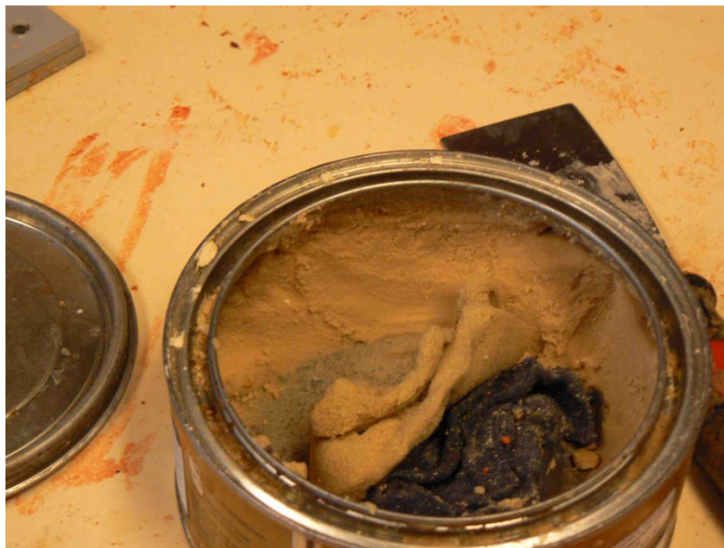
Figure 3.2: Wax Lubricant with Sponge and Paint Scraper used for Cleaning
