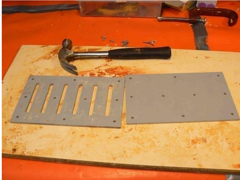
Figure 3.1: The Two PVC Plates that make up a Mould Set
