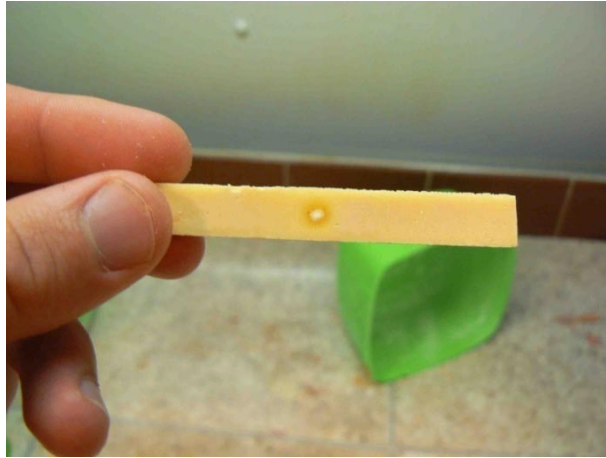
Figure 3.6: Glass clump in Final Specimen due to poor mixing
