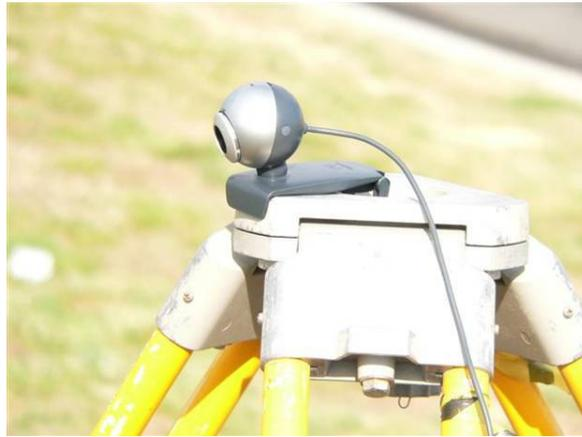
Figure 3.12 – A web camera erected on a spare tripod.
