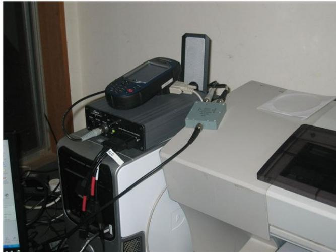
Figure 3.5 – ProMark3 connected to Rojone Splitter Box and Ashtech Dual Frequency Receiver.
