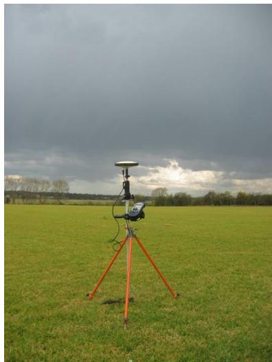
Figure 4.1 – ProMark3 Rover setup on a Permanent Mark 67533 buried in the ground.
