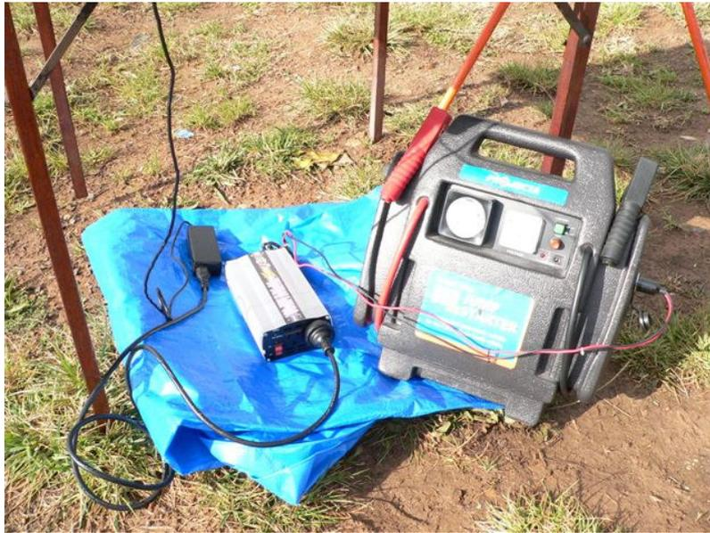
Figure 3.11 - Projecta 12V 17Ah Sealed AGM Portable Battery with 300W DC – AC power inverter
