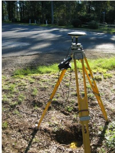
Figure 3.4 – Typical Field setup showing ProMark3 with 1m long antenna cable.
