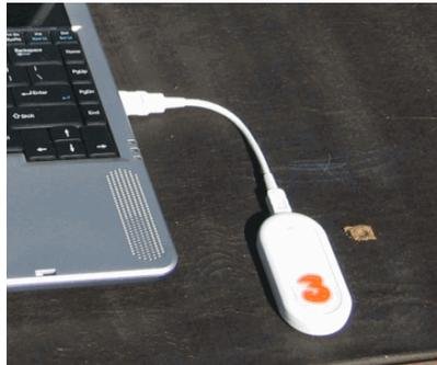
Figure 3.10 – 3 Mobile Broadband Modem connecting to a laptop computer USB port.
