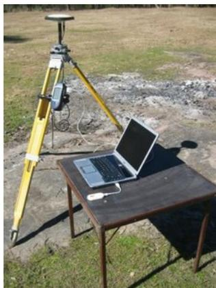
Figure 3.9 – A basic design for a portable field GNSS network solution using the ProMark3.
