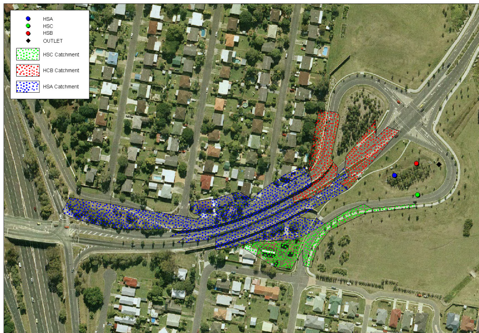
Figure 4.2 Catchments discharging into the Hoyland Street bioretention system
