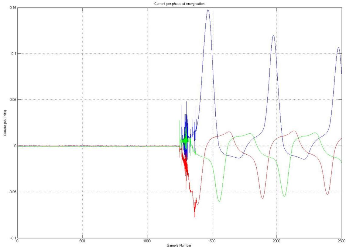
Figure 9 - Three Phase Energisation of a test transformer (Current)
