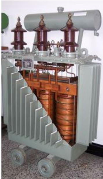
Figure 6 - Internal design of a power transformer
