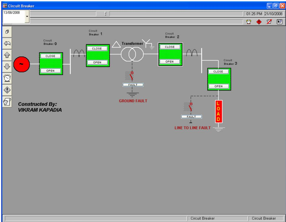
Figure 17 - SCADA interface to the test rack system
