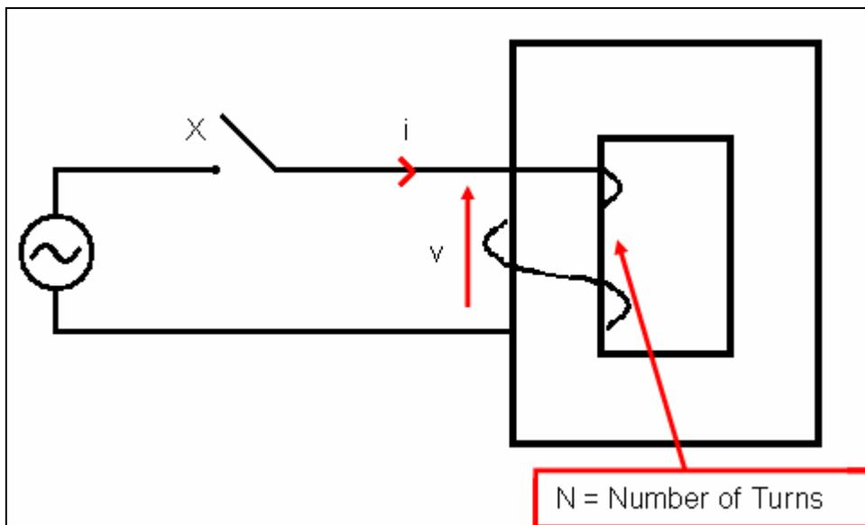
Figure 1 - Transformer Model No-Load
