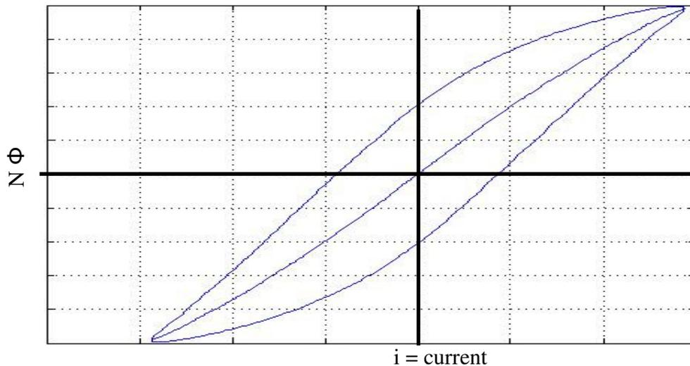
Figure 3 - Transformer Hysteresis Loop
