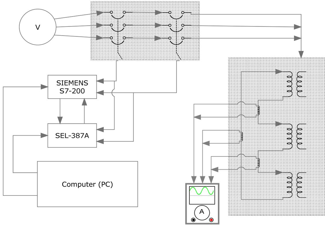
Figure 18 - Test Rack design
