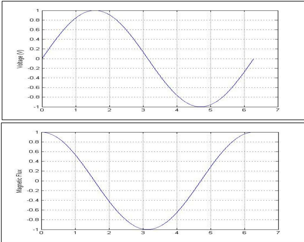
Figure 2 - Steady State Voltage and Magnetic Flux Waveforms
