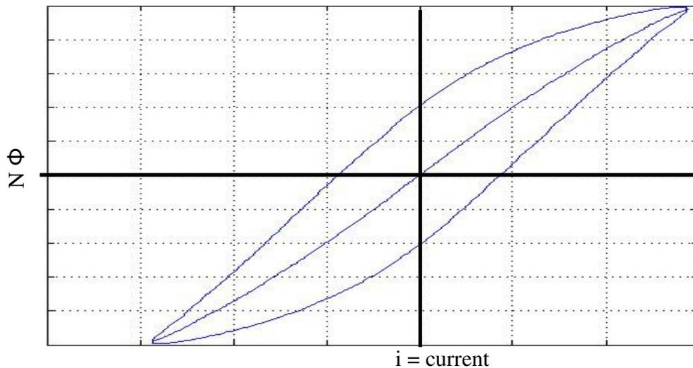
Figure 13 - Transformer Hysteresis Loop
