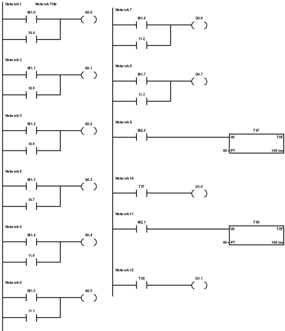
Figure 16 - PLC Ladder Diagram for the Circuit Breaker
