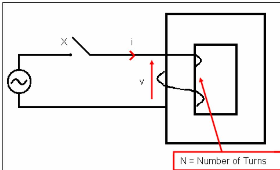
Figure 11 - Transformer Model No-Load
