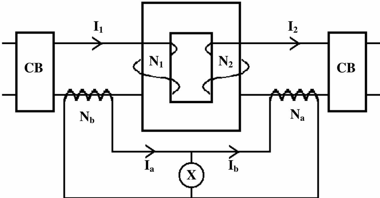
Figure 7 - Simplistic Differential Protection Schematic
