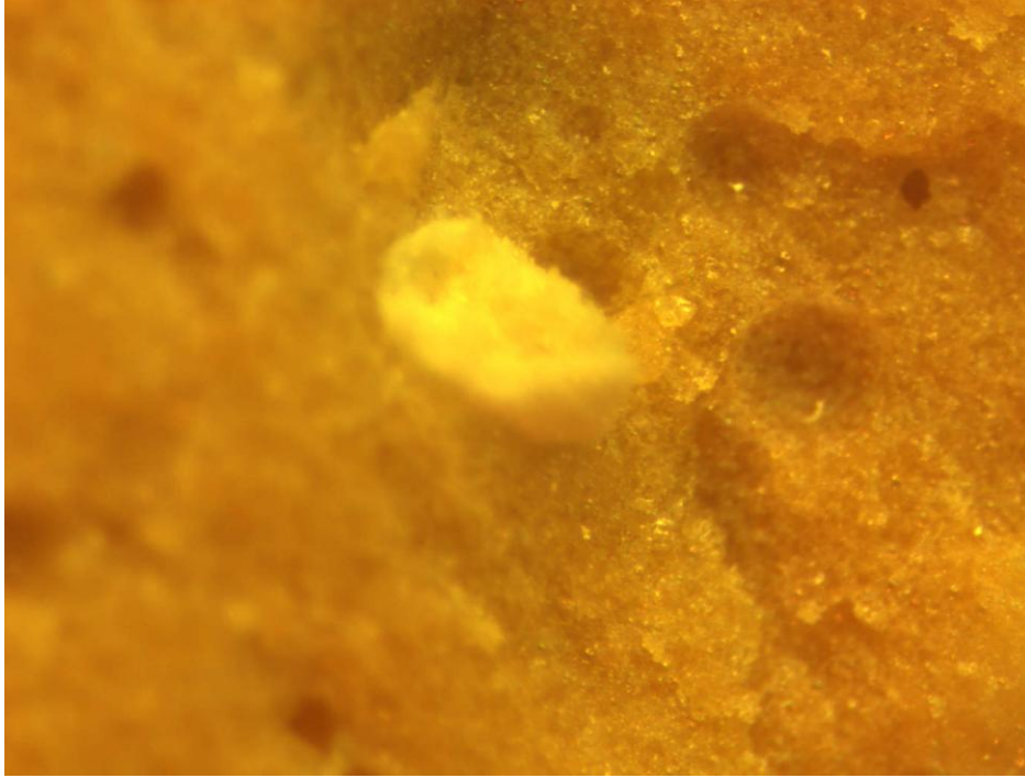
Figure 4-10 Microscopic view of specimen, with glass powder at 140 times magnification
