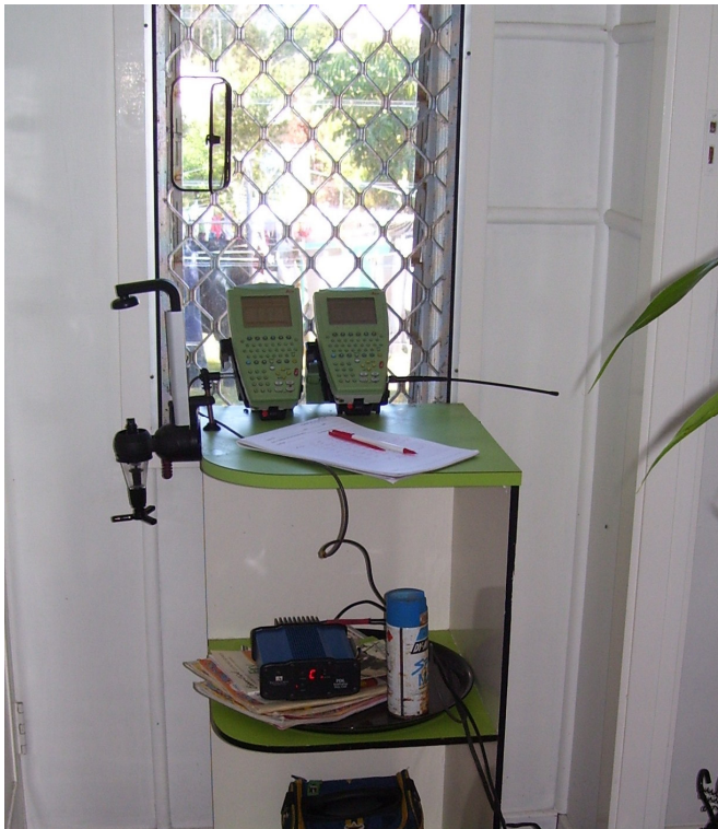
Figure 3.4.2 Controller setup with a Bluetooth connection
