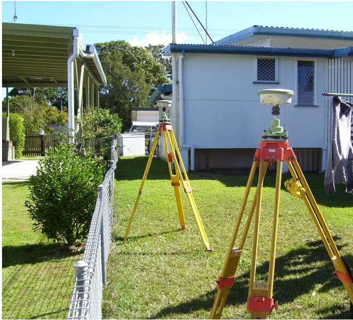
Figure 3.4.1 Base and Rover set up for data collection
