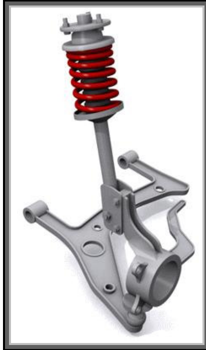
Figure 2.5.2 – McPherson strut suspension.
