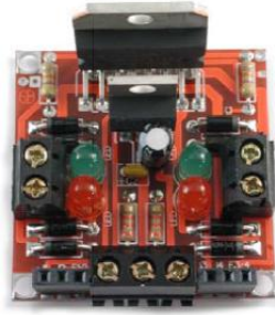
Figure 3.14 L298 motor driver PCB (Solarbotics)
