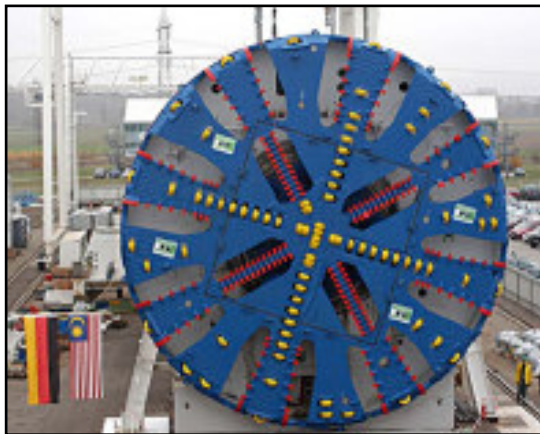
Figure 3g: Slurry Shield TBM at SMART Project
