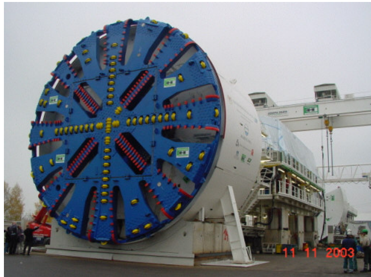
Figure 4d: TUAH TBM
