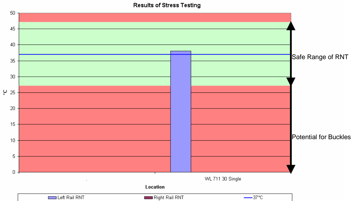
Figure 4.5 A chart of the results in table 4.5, shows the safe range of RNT about the 37°C DNT
