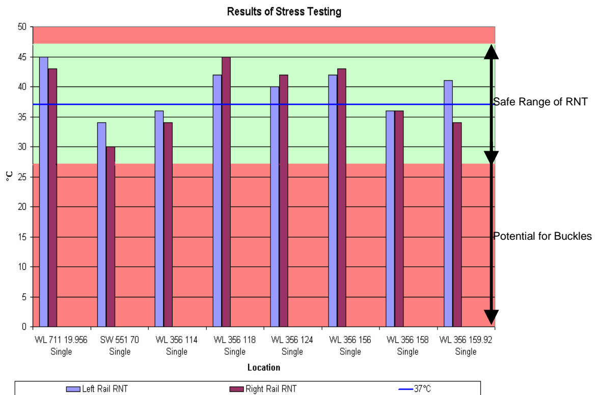
Figure 4.8 A chart of the results in table 4.7, shows the safe range of RNT about the 37°C DNT
