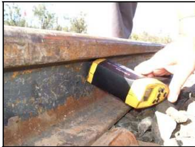
Figure 6 - Measuring Rail Temperature
