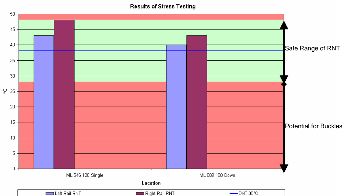
Figure 4.7 A chart of the results in table 4.6, shows the safe range of RNT about the 38°C DNT
