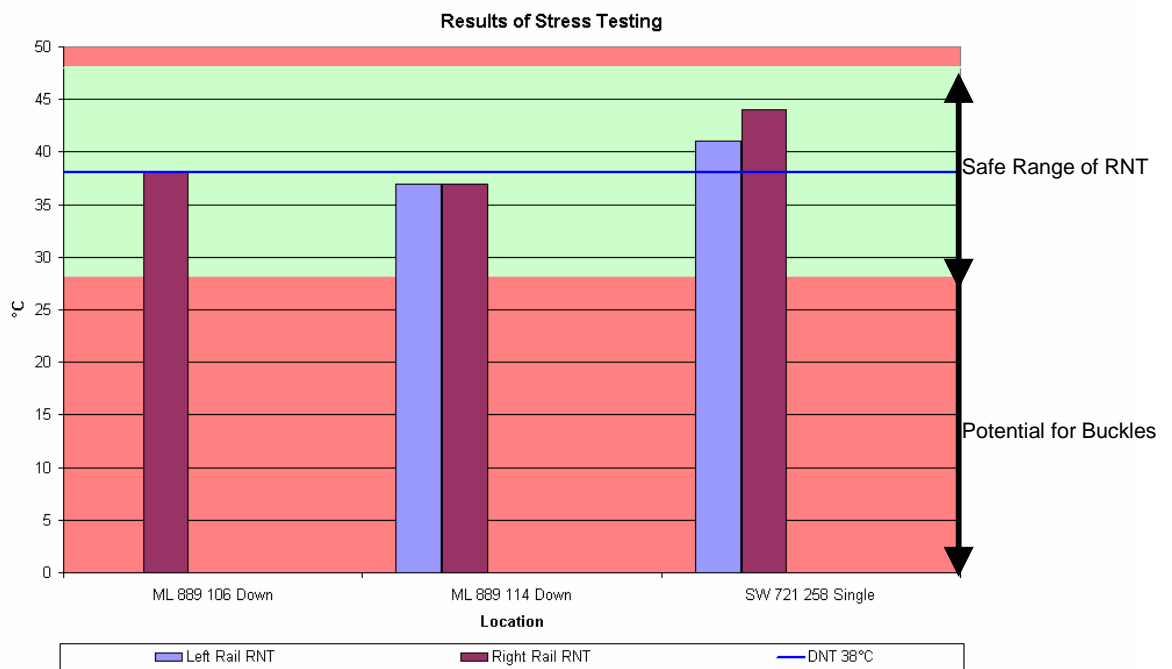
Figure 4.4 A chart of the results in table 4.5, shows the safe range of RNT about the 38°C DNT
