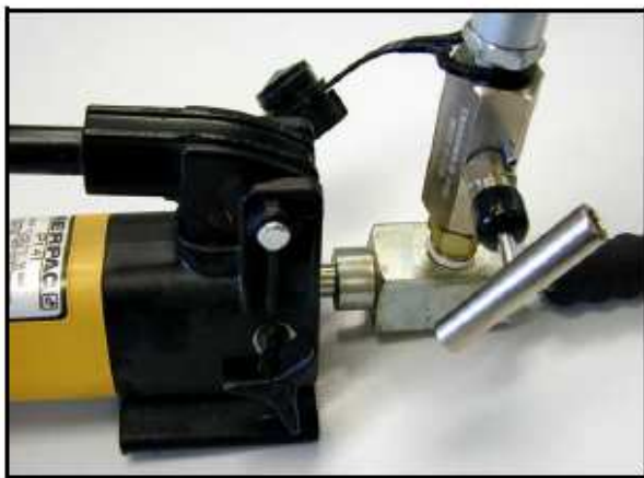
Figure 5: Regulating and Gauge Isolation Valves
