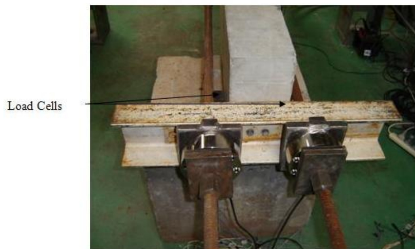
Figure 4.17: Load Cells in Position for Initial Prestressing
