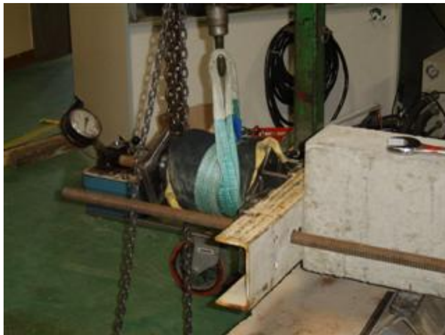
Figure 4.18: Hydraulic Jack and Prestressing Apparatus
