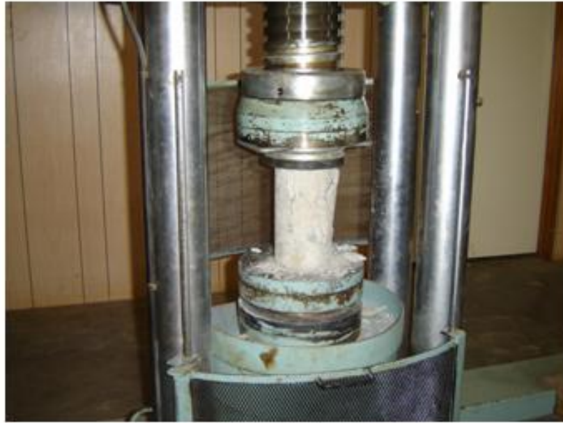
Figure 4.9: Compression Testing of the Concrete Cylinders in the Avery Machine
