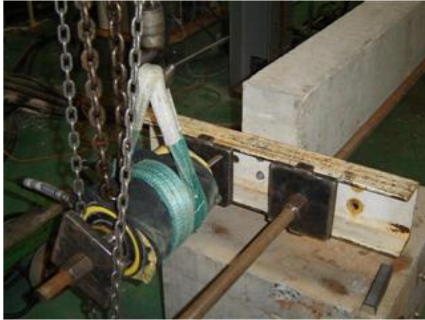
Figure 3.13: Prestress Anchorage and Jacking System
