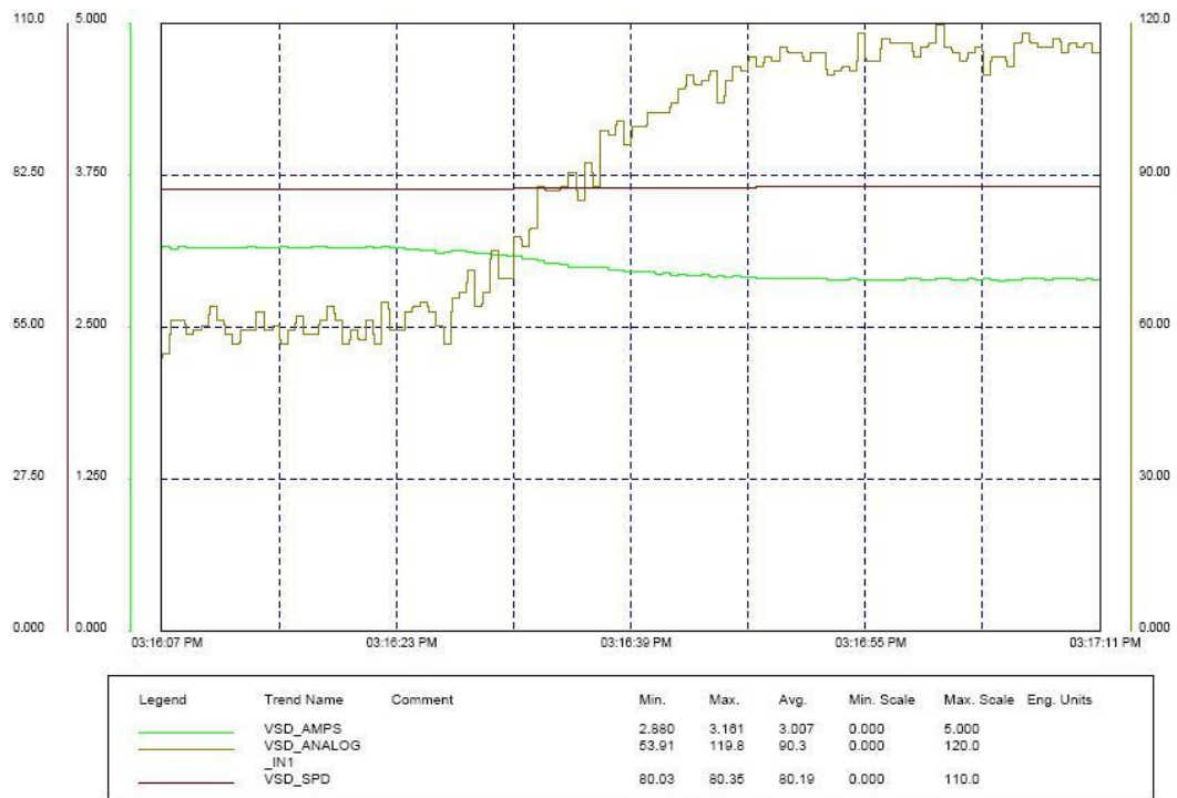
Figure 4.8: Plot of Pressure and Motor Current when speed is held at 80%
