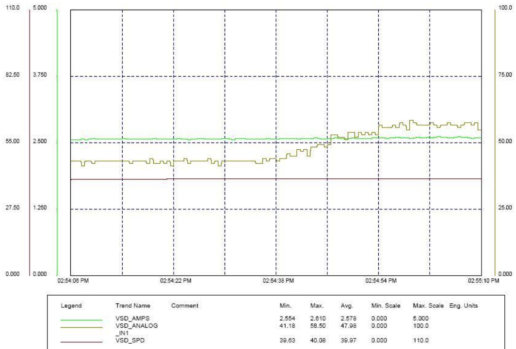
Figure 4.4: Plot of Pressure and Motor Current when speed is held at 40%
