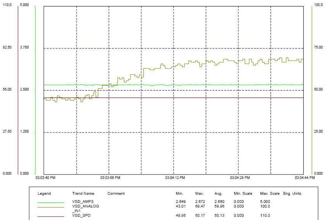
Figure 4.5: Plot of Pressure and Motor Current when speed is held at 50%
