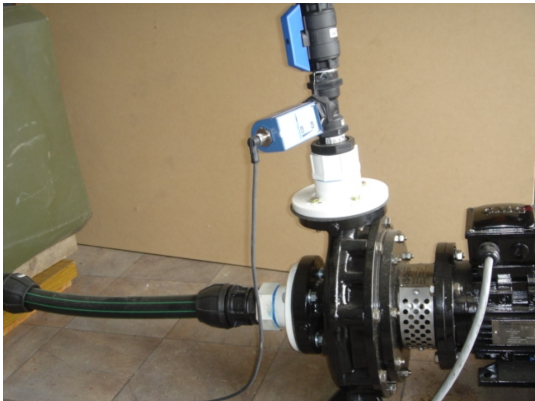
Figure 3.2: This Photograph is of Closed Loop Testing System's Pump and Pressure Transmitter
