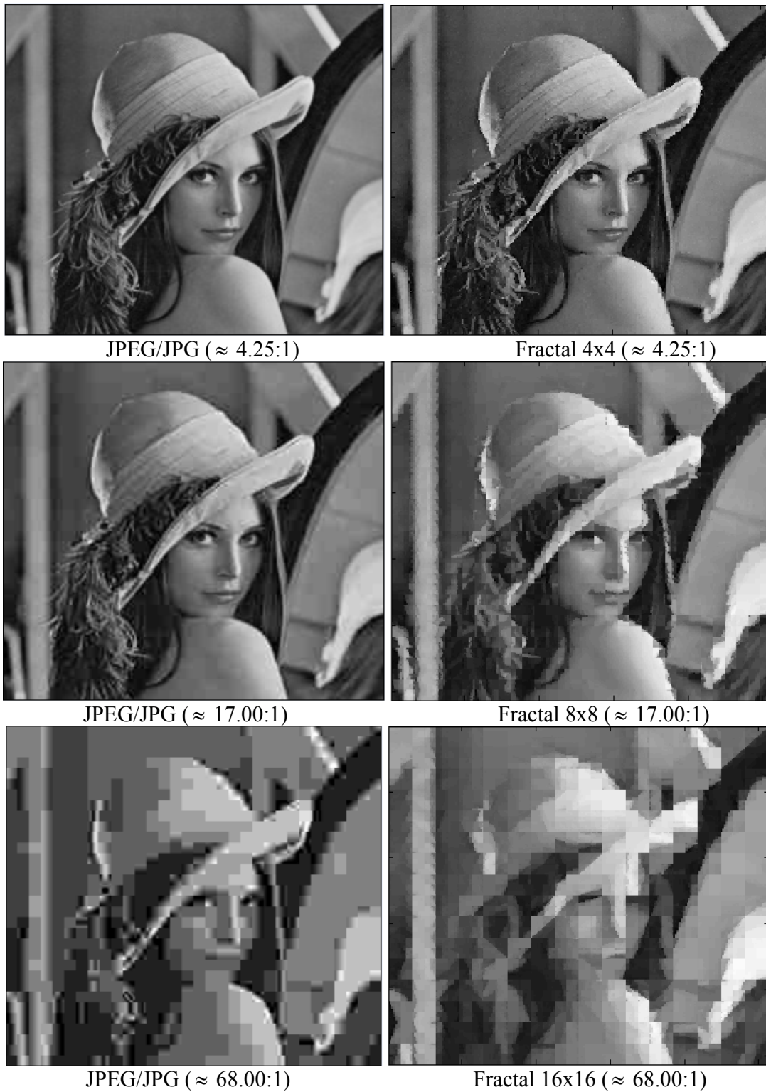
Figure 4.8: Lena image decompressed using fractal-based compression and JPEG/JPG with different compression ratios.
