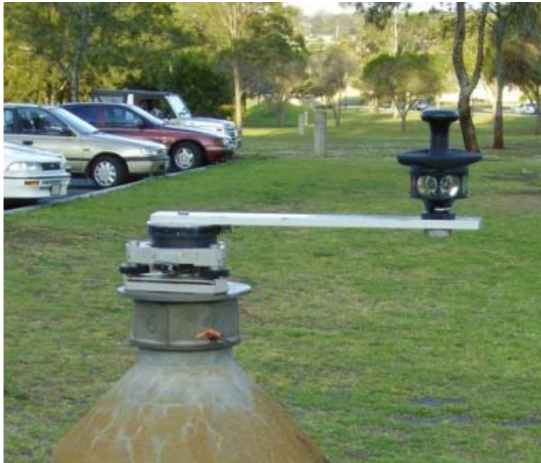
Figure 3.4: Circular Path target assembly.
