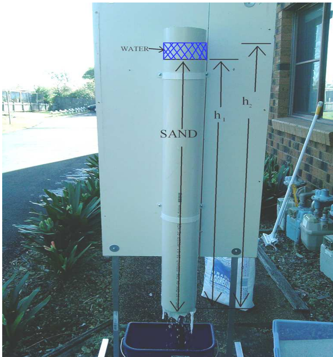
Figure 3.5.1 -Permeability experiment basic overview
