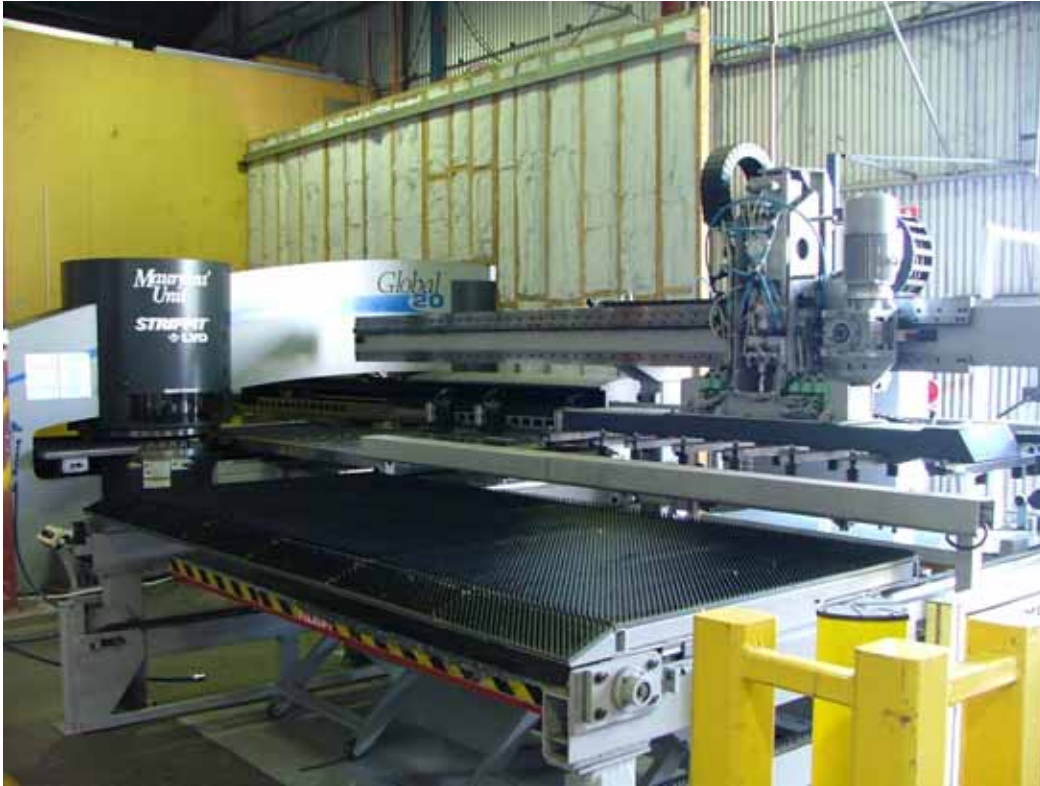
Figure 7.9 Global 2.0, a very high capacity punching machine.
