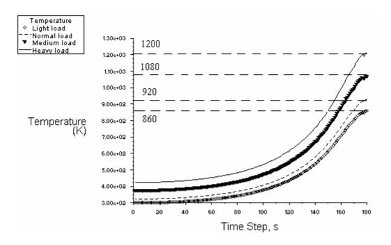
Figure 6.8 - Temperature Distribution for Different Load Conditions for CR=19.3:1
