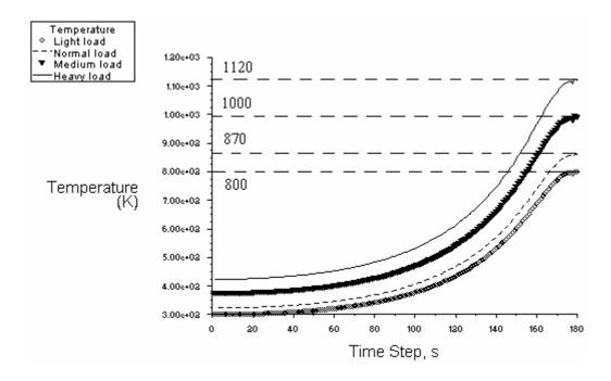
Figure 6.11 - Temperature Distribution for Different Load Conditions for CR = 16.6:1
