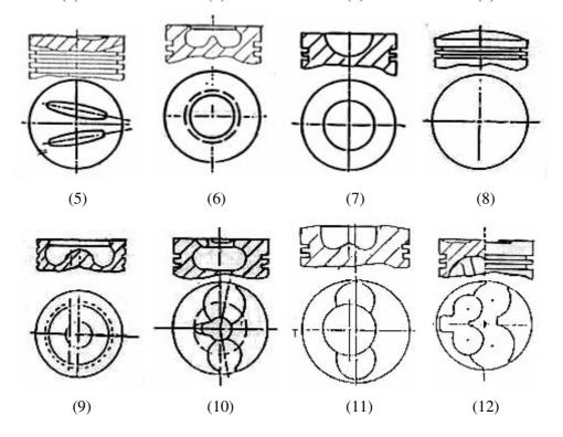
Figure 3.2 - Various Shapes of Piston Crown (KVR BMC Pistons Limited 2004 <a href="http://www.kvrbmc.com/shape\_pis.htm">http://www.kvrbmc.com/shape\_pis.htm</a>)
