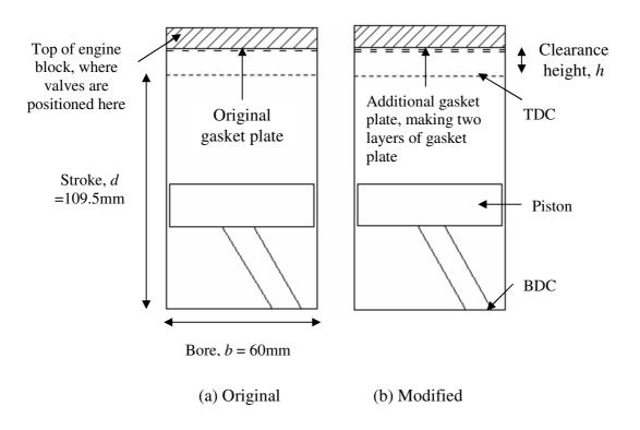
Figure 5.2 – Additional Plate to Increase Clearance Volume
