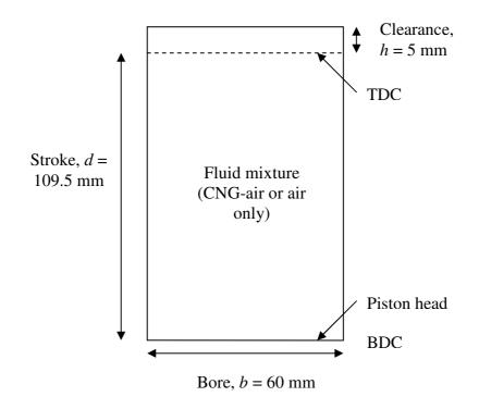
Figure 5.1 – Simulation Model
