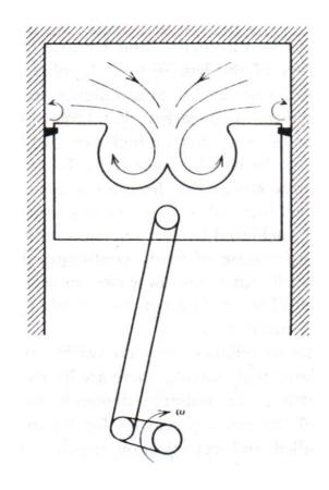
Figure 3.5 – Swirl Generated by Squish Motion about a Circumferential Axis in Piston Bowl (Ferguson 1986, p.299)
