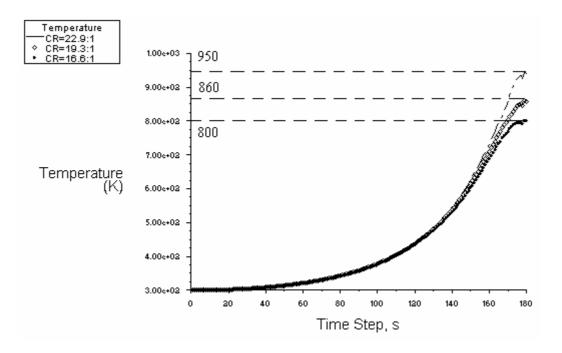
Figure 6.5 - Temperature Distribution for Different Compression Ratios (CR)
