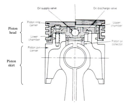
Figure 3.1 - Structure of Piston (Ferguson 1986, p. 46)
