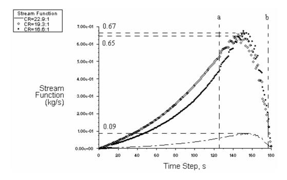
Figure 6.6 – Stream Function Distribution for Different Compression Ratios (CR)
