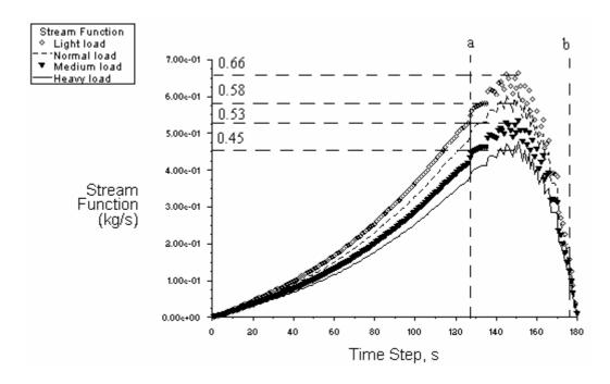
Figure 6.9 – Stream Function Distribution for Different Load Conditions for CR = 19.3:1
