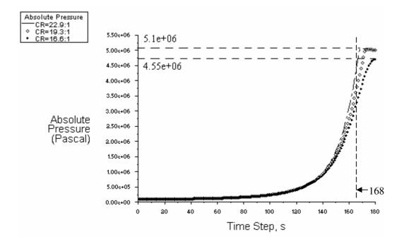
Figure 6.4 - Pressure Distribution for Different Compression Ratios (CR)
