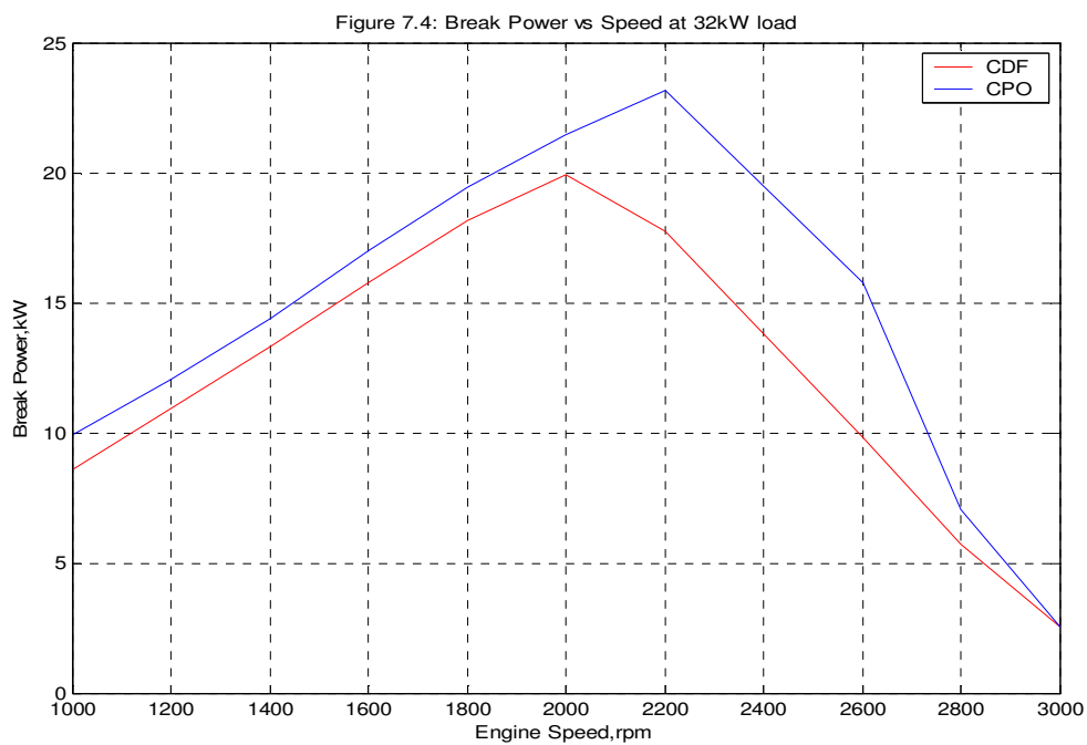
Figure 7.4 Brake Power vs. Speed at 32kW load
