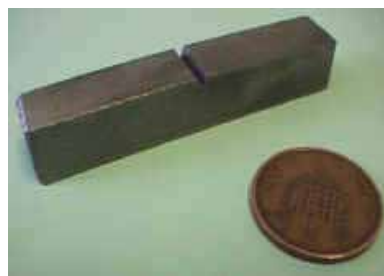
Figure 4.2: A Charpy test specimen
