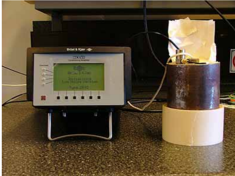
Figure 4.7: Charger Amplifier (Left) and impact tup (Right)
