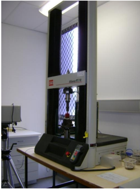
Figure 3.9: MTS Alliance (flexural and impact toughness testing machine (10 kN).
