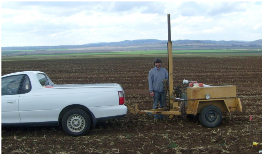
Figure 3-3 Soil core rig attached to utility
