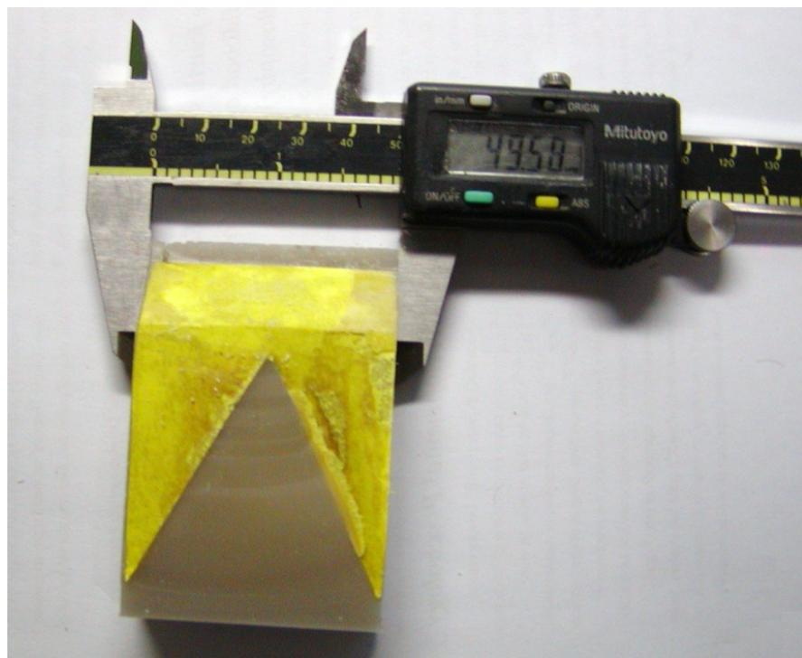
**Figure 10.7: Taking measurement of the test specimen using digital vernier callipers.**
