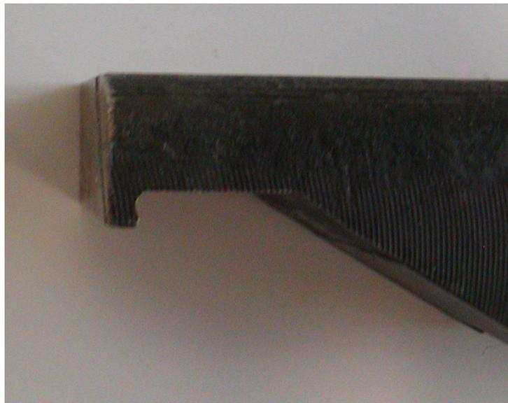
**Figure 10.5: Gripper used in MTS 810 Material Testing System**
