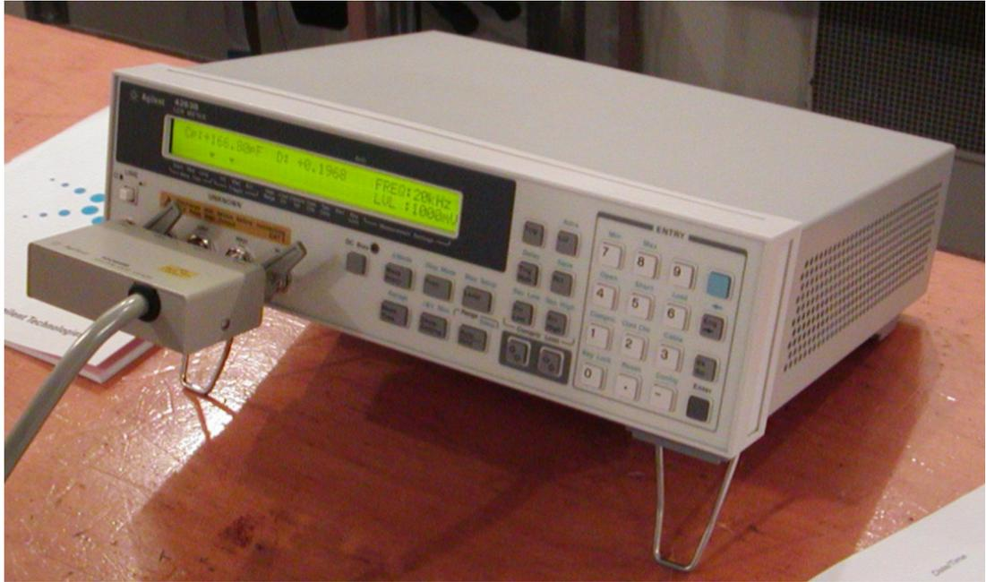
Figure 11.7: Agilent 4263B LCR Meter.
