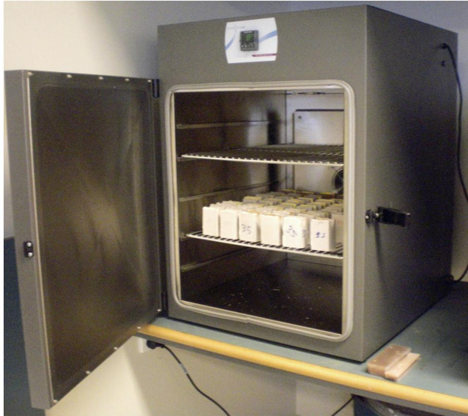
**Figure 3.7: The Steridium laboratory oven used for the post-curing process of the specimens**
