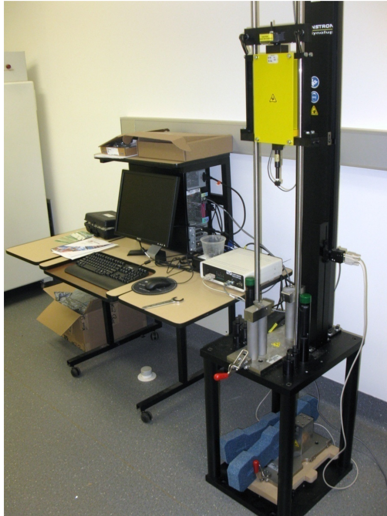
Figure 24 - Instron Dynatup M14-15162 Impulse Impact Testing System used in impact tests
