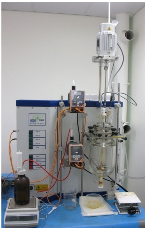
Figure 14 - Mettler Toledo Labmax used in synthesis of resin
