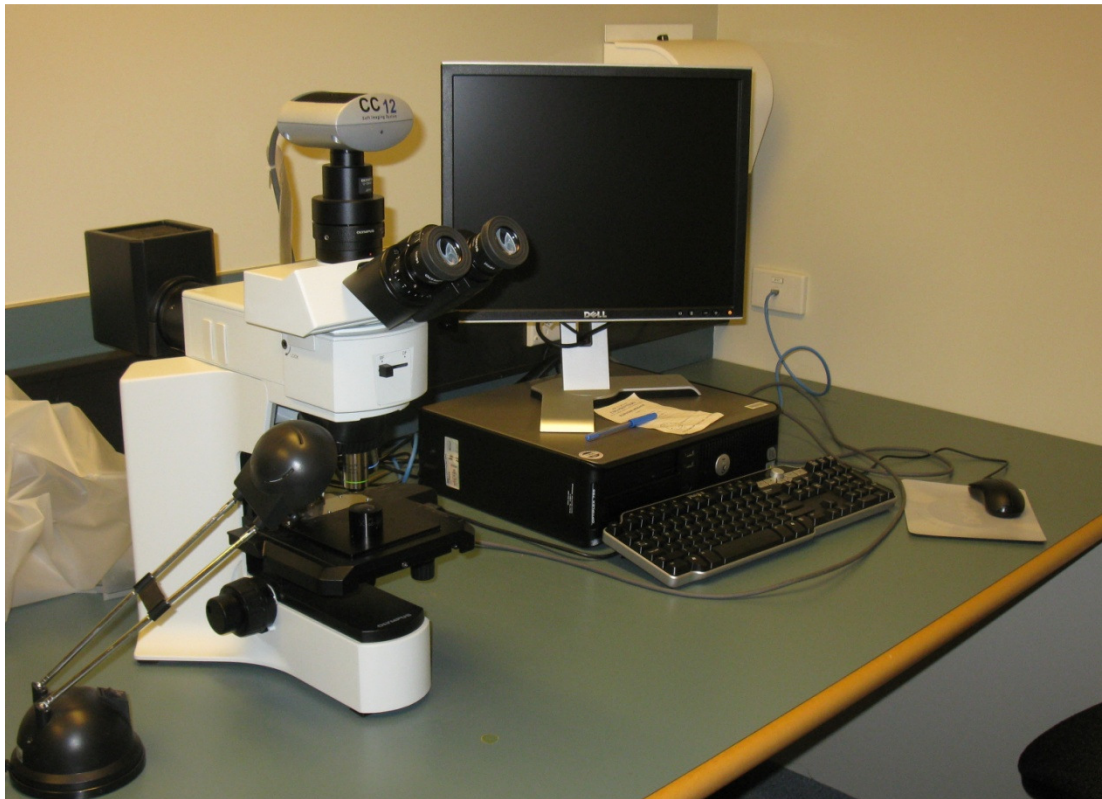
Figure 27 - Olympus BX41M optical microscope used in analysis
