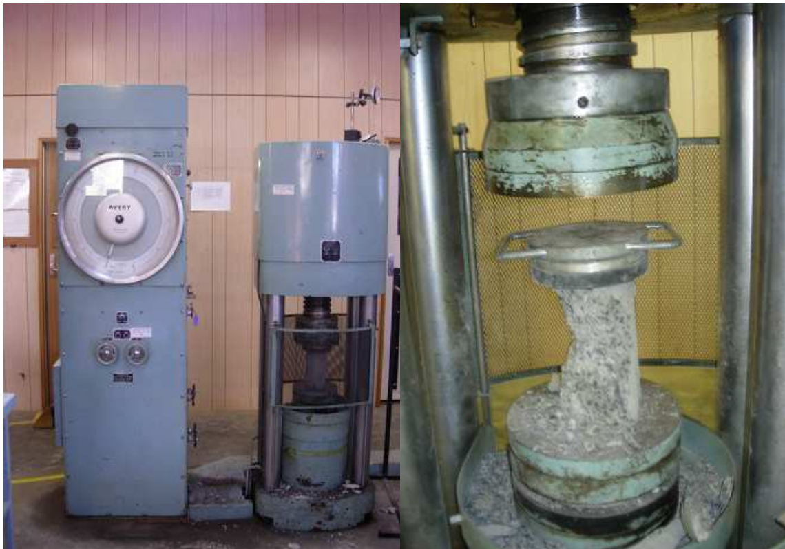
Figure 3.16 (Left) Cement compression testing machine.(right) close up of the compression mechanism.
