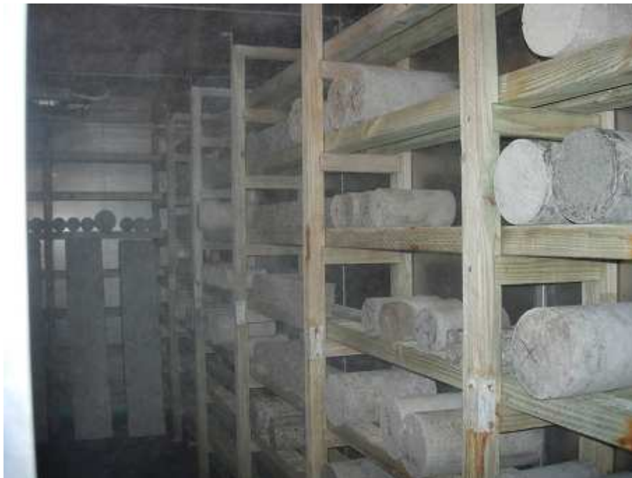
Figure 3.15 inside the humidity room
