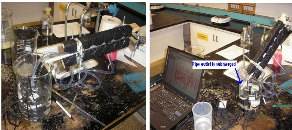
Figure 3.21 (left) pipe position for Test A-G (right) submerged pipe position for Test F – onwards.
