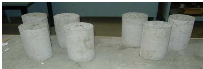
Figure 3.14 (left) Type of mould used to make cylinders (right) Cylinders after they were cured for 31 days.
