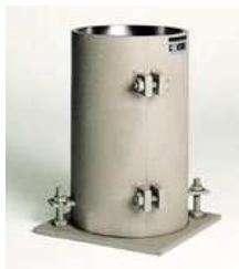
Figure 3.14 (left) Type of mould used to make cylinders (right) Cylinders after they were cured for 31 days.
