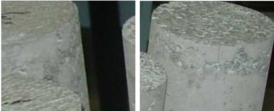
Figure 4.32 Cylinders that weren't packed as well as could have been.
