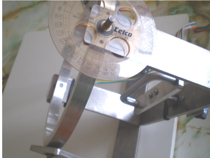
FIGURE 6-5: PROTRACTOR MOUNTED ON THE DEVICE FOR POSITION TESTING.
