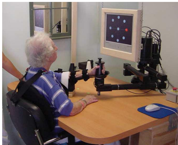
FIGURE 2-14: THE MIT-MANUS SET UP IN A HOSPITAL DURING CLINICAL TRIALS (KREBS ET AL. 2007).
