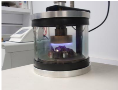
Figure 3.4 Gold coating specimens
