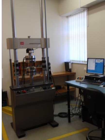
Figure 3.3 Tensile Machine, with outputs read by the computer
