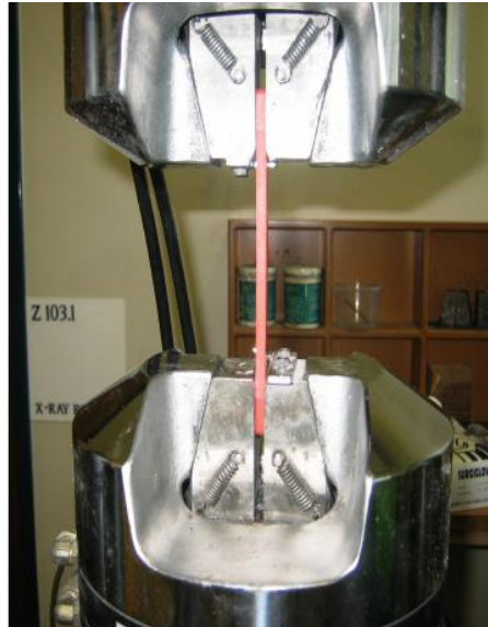
Figure 3.2 Specimen held in the hydraulic wedge grips of Tensile Testing Machine (Ready for testing)
