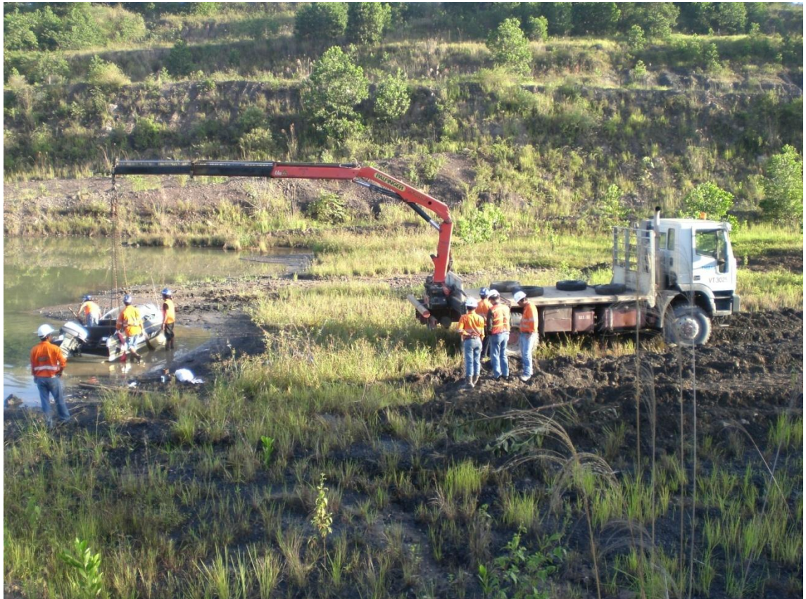
Figure 3.7 Iveco Flat Bed Truck Lifting the Sapu Lidi to Waters Edge
