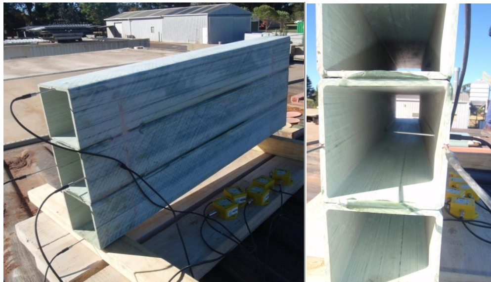
Figure 3.13: The experimental test setup for bonded pultrusion beam.
