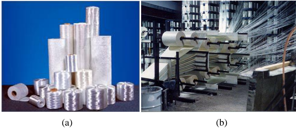
Figure 2.11: (a) Various sizes and forms of E-glass as manufactured ( ), (b) E-glass used in a pultrusion machine during material manufacture (Bedford Reinforced Plastics Inc. 2009).
