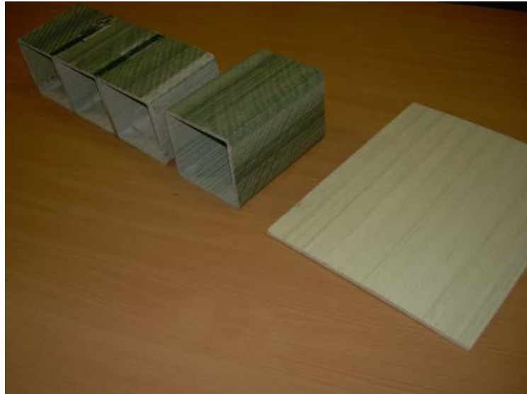
Figure 2.14: 375 mm x125 mm web, 125 mm x125 mm pultrusion and 300 mm x 6 mm pultrusion (Wagners CFT 2008).
