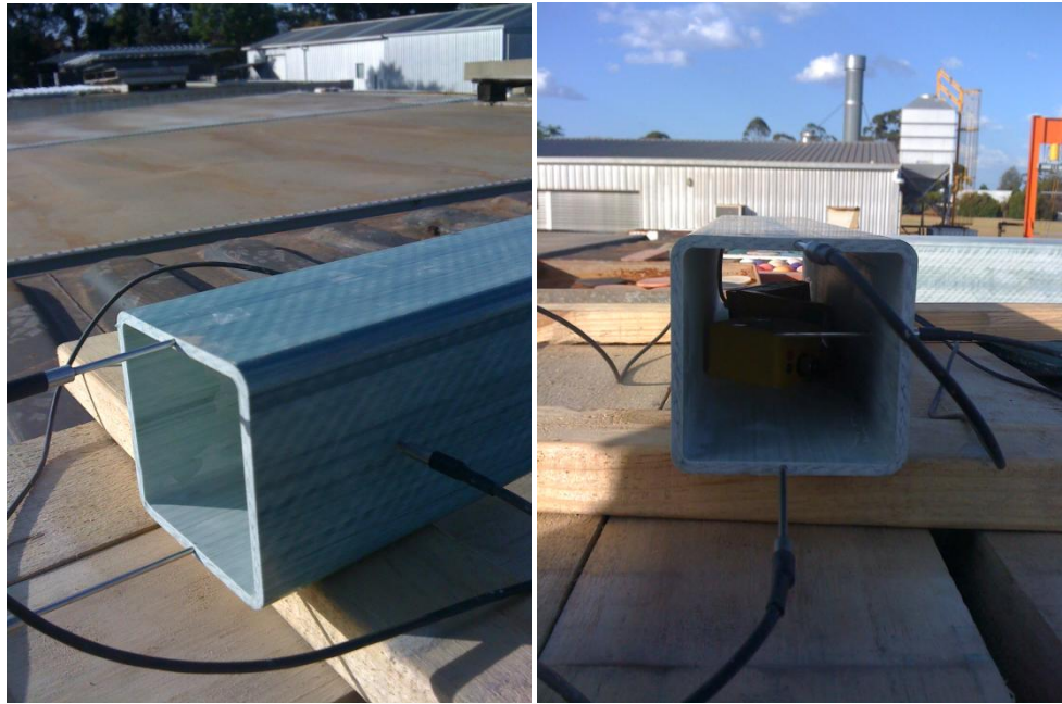
Figure 3.14: The experimental test setup for single pultrusion member.
