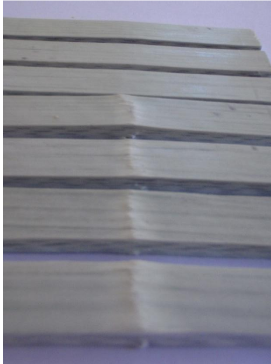
Figure 4.4: Bottom surface of samples tested from 20°C (closest) to 105°C (farthest).
