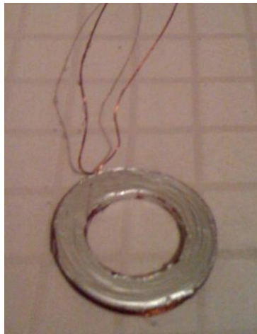
Figure 5-29: Coil after removal from the former.
