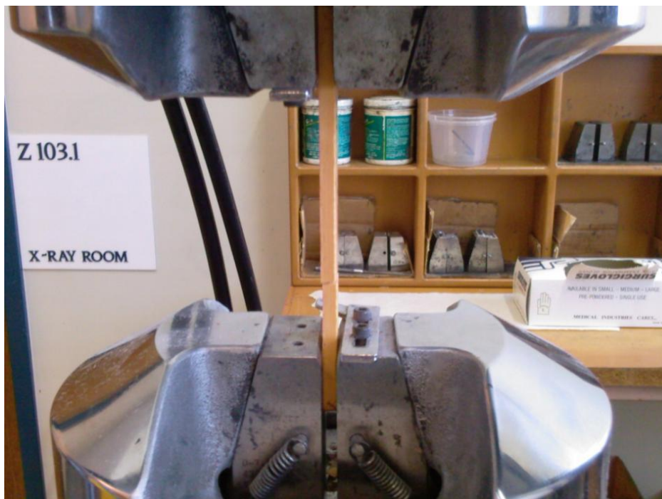
Figure 4-1 Test piece loaded in the tensile testing machine
