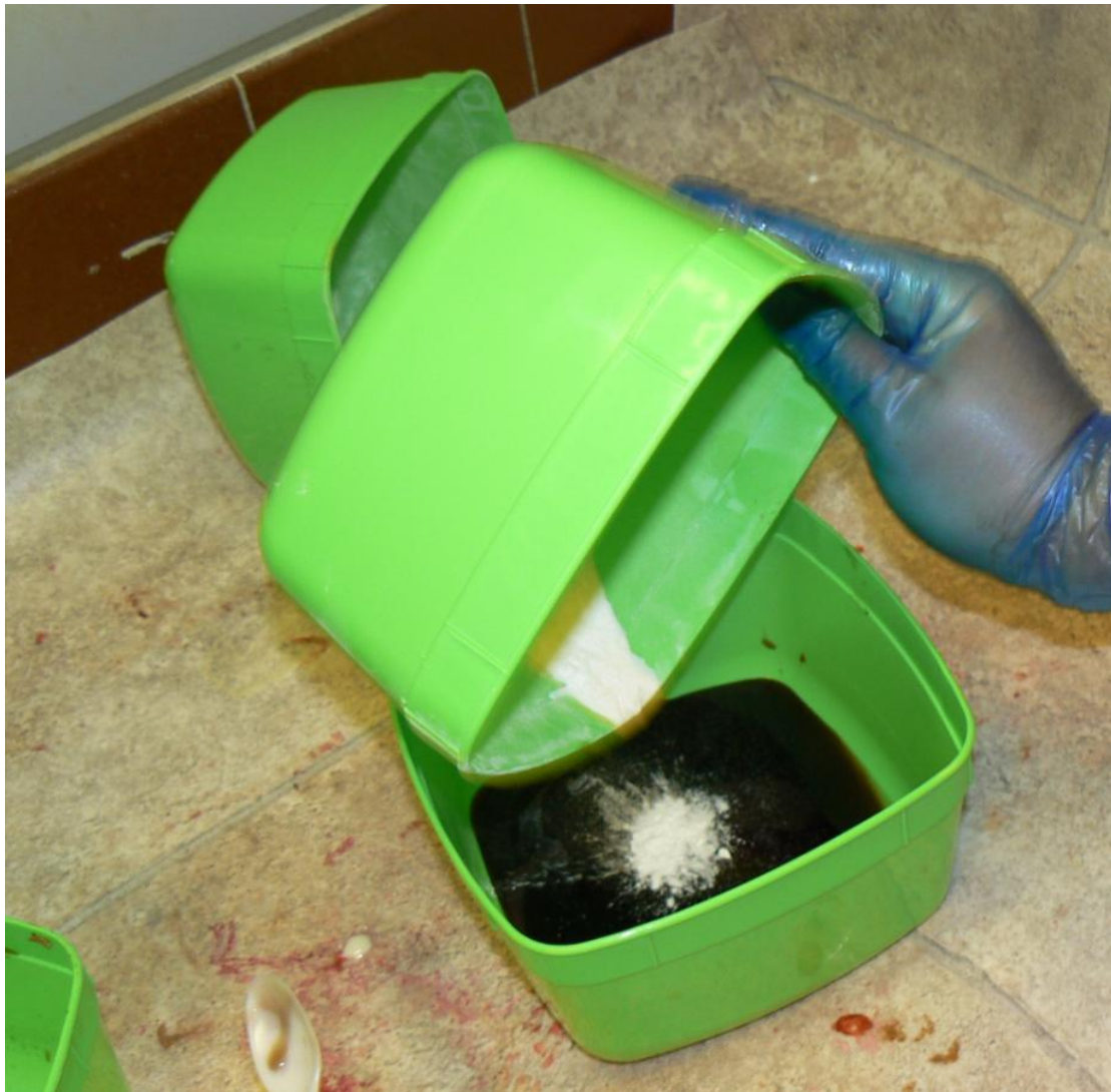
Figure 3-2 illustrates the glass being added to phenolic resin
