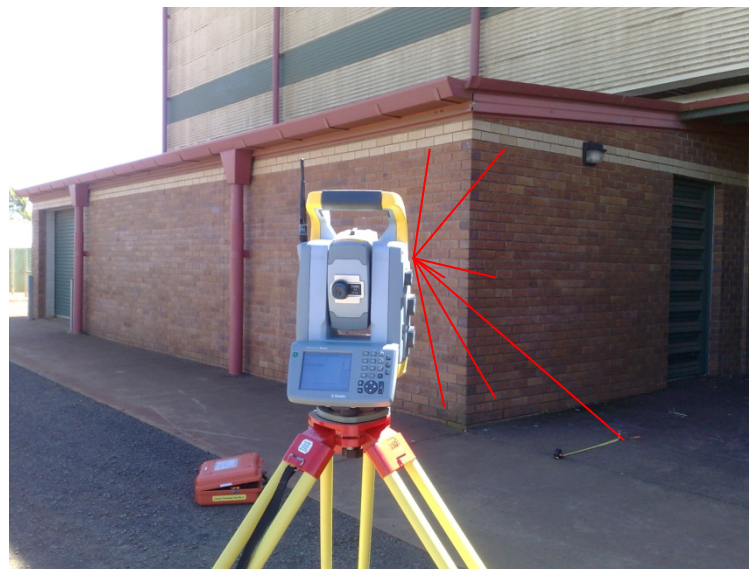
Figure 3.7: Volumetric Test, Building Encroachment.
