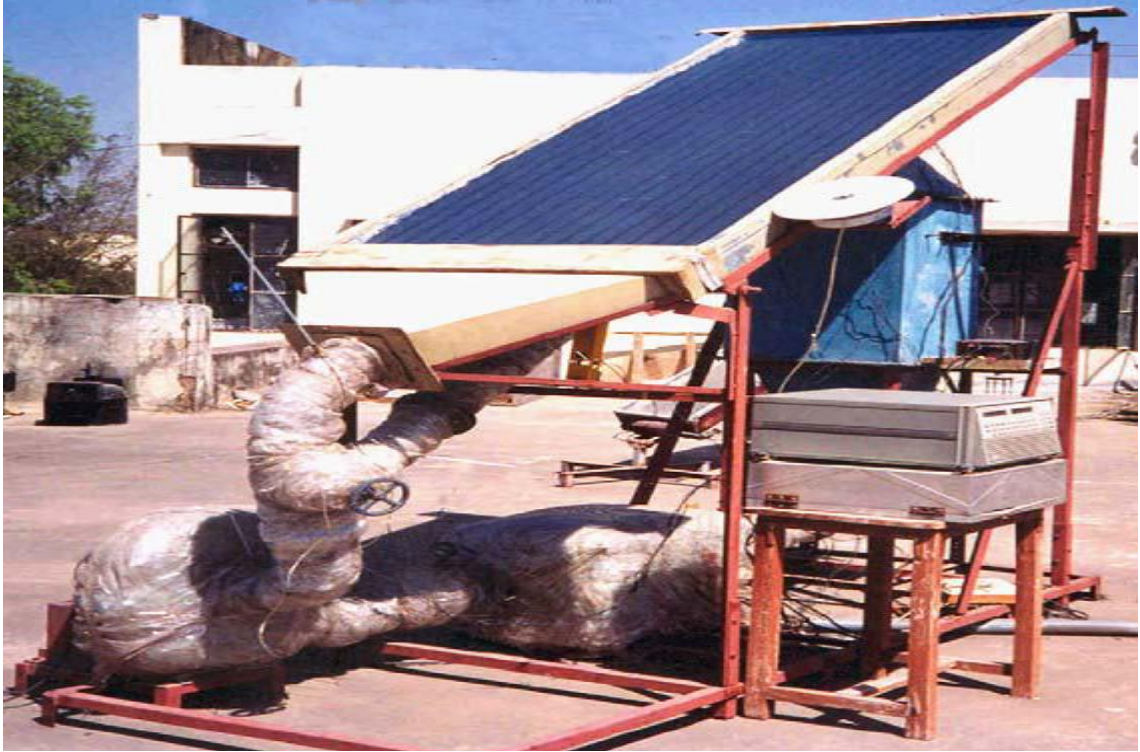
Figure 47 - Sarsavadia developed a solar assisted forced convection dryer for dehydration of onions slices for the controlled condition.
