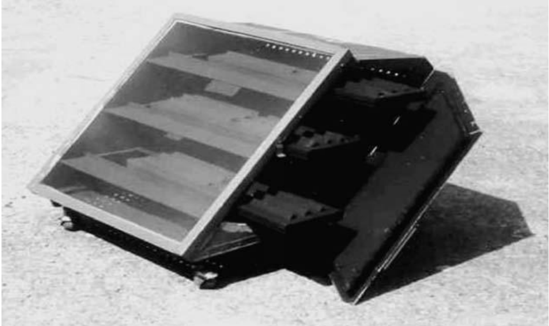
Figure 39 - Singh et.al developed a multi- shelf domestic solar dryer for drying various products.
