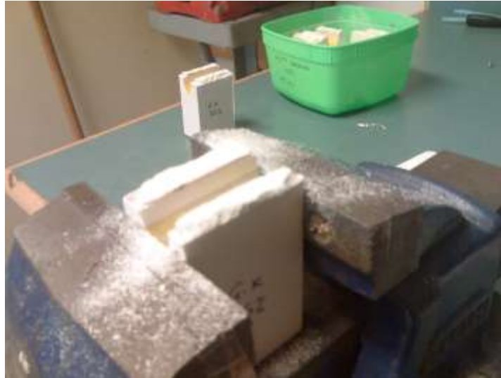
Figure 3.6: Filing down a specimen to required length
