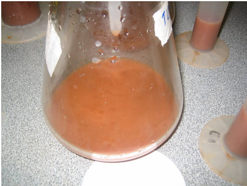
Figure 5.8: Visible colloids present in Toowoomba soil PLD drainage water sample
