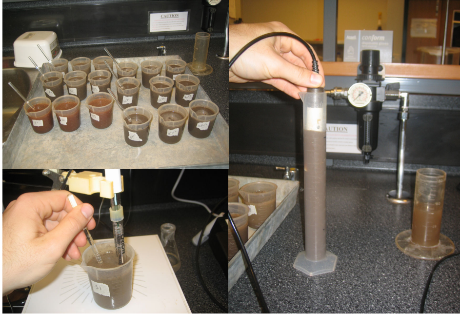
Figure 3.3: Performing 1:5 soil-water pH & EC experiment
