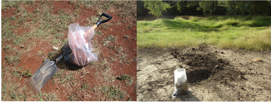
Figure 3.1: Method of soil sample collection
